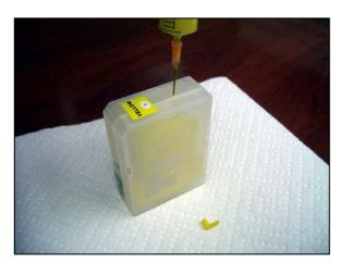
Refill the syringe and continue injecting ink into the cartridge until the cartridge is full. It will take nearly three complete syringes full of ink to fill the cartridge. Use paper towel to wipe any ink from the surface of the cartridge, and return any ink in the syringe back to the correct color bottle.
