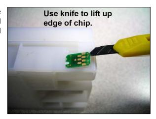
Take the refillable cartridge that corresponds to the color of the original chip you have just removed, and remove the bridge chip from the cartridge. Removing the bridge chip is very simple – simply use a small screw driver to lever up the plastic at the end of the bridge chip as in this picture. Once you have levered up the end of the plastic, the bridge chip can be completely removed from the cartridge.
