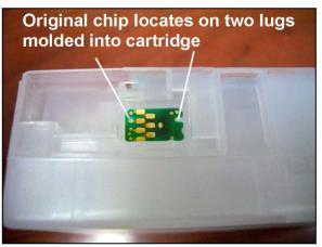
Now take the bridge chip and gently push it down on top of the original chip. The bridge chip will snap into place flush with the top surface of the cartridge, as in this picture. The bridge chip has spring loaded pins that line up with the gold contacts on the original chip below. Repeat this process of removing original chips and installing them beneath the bridge chips for on any of the other colors you are going to install at this time.
