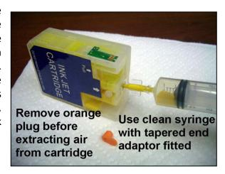
Replace the orange rubber plug over the air port before moving the cartridge. You can now top up the cartridge with ink again as in step 2 above, if you wish. Wash out the syringe and adaptor using water under a faucet. The cartridge is now ready for use. Repeat steps 1, 2, and 3 with any cartridges you want to fill and use at this time.
