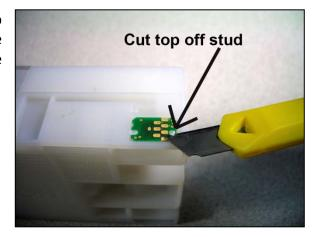
Once you have trimmed off the top of the plastic stud, use the knife to lift up the edge of the chip. The chip can now be pulled off the original cartridge. Try to avoid touching the gold contacts on the chip when handling it.
