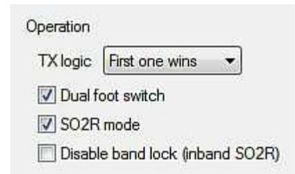
**Dual foot switch:** MK2R has two foot switch inputs.
