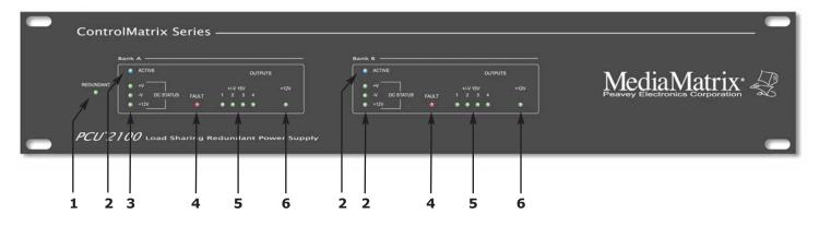
**1. REDUNDANT MODE LED** Single color LED (Yellow) indicates that the PCU 2100 is operating in Redundant Mode. If the unit is operating in Dual Mode, this LED will not be illuminated.
