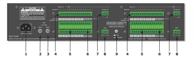
**1. IEC POWER CONNECTOR** Standard IEC power receptacle for connecting AC Mains supply. Use only the supplied cable.
