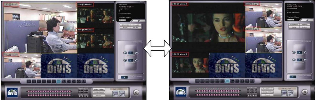
At the connection of DiViS Net software, connected cameras will be positioned in order of camera numbers. It is possible to relocate the camera position to the desired location by left clicking on the image that needs to be relocated, dragging it to the new position, and releasing the left mouse button.
