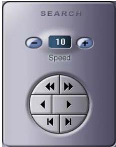
**Search Tools:** Buttons in upper line works for fast rewind (left directional arrow) and fast forward (right directional arrow). Buttons in middle line activate the normal playing back in forward and reverse but the speed can be adjusted by controlling ( - ),( + ) tabs on the top. The buttons in lower line give playback frame by frame, forward or reverse.
