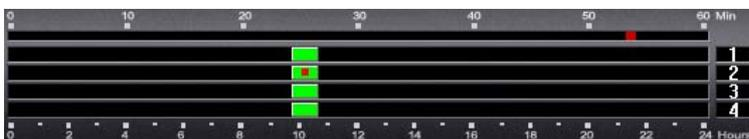
: The camera number is shown on the right in a vertically descending order in blocks of four, the hour is shown on the bottom with each hour represented by one green block, and the minute is shown on the top, with each minute represented by a smaller green block. The user can search for a recording at a specific time by clicking on a specific hour block on a specific camera number row and a specific minute block afterwards (as shown above).
