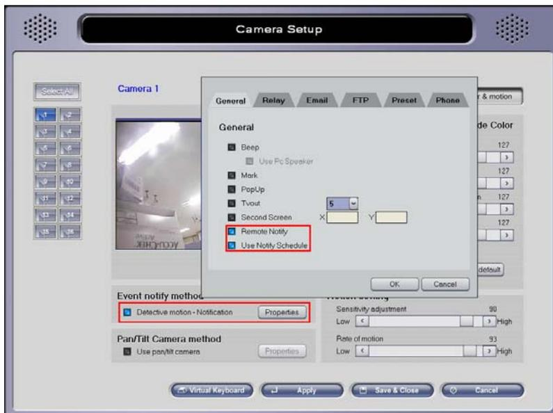
Exit “System Setup” and enter “Color & Motion” configuration under “Camera Setup.” Check “Detective motion – Notification”. Click on “Properties”, and check “Remote Notify” to send notifications when an event occurs. Check “Use Notify Schedule” to utilize the schedule to notify the DiViS Net. If selected, notification schedule on the following page must be configured.
