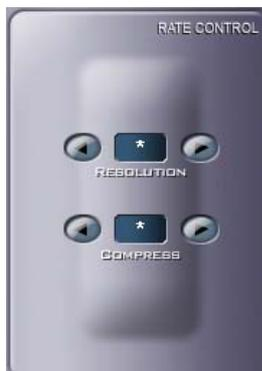
: Compression Rate can be adjusted between 10 ~ 90 to enhance the transmission speed (\* for default compression rate). Lower compression rate will provide faster transmission. Resolution can be selected among 1/2, 1/4, or 1/8 (\* for default resolution), and lower resolution provides faster transmission speed. Compression rate and resolution adjusted here are not changing actual resolution and compression rate recorded on the server.
