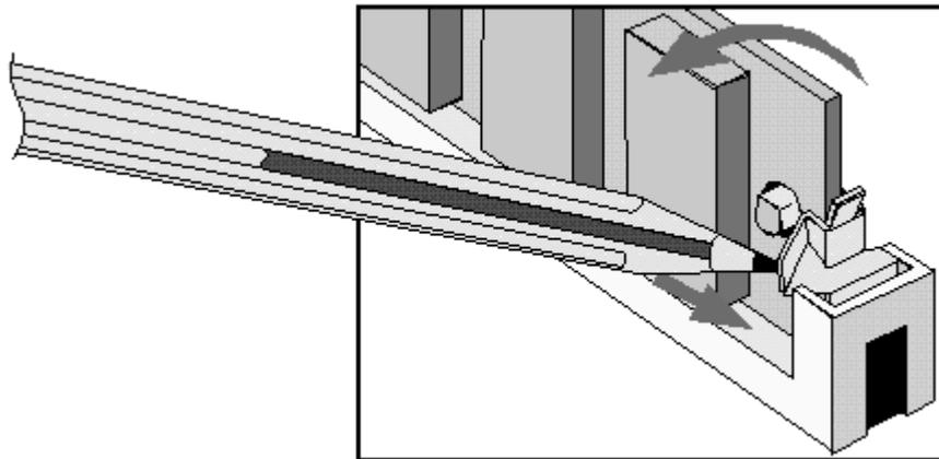
**Release the retaining clip and pull the module forward and out of the socket**
