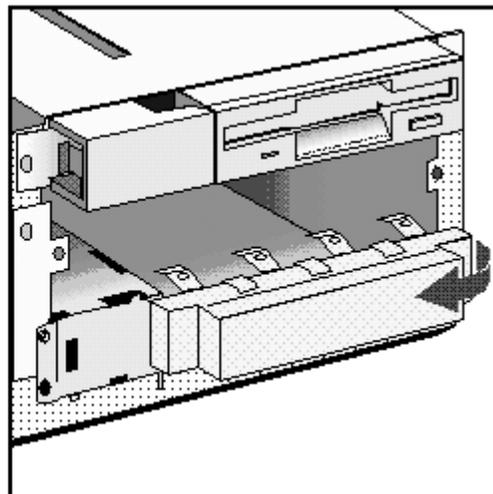
6 Remove the side bracket from the bottom shelf and store it in a safe place.
