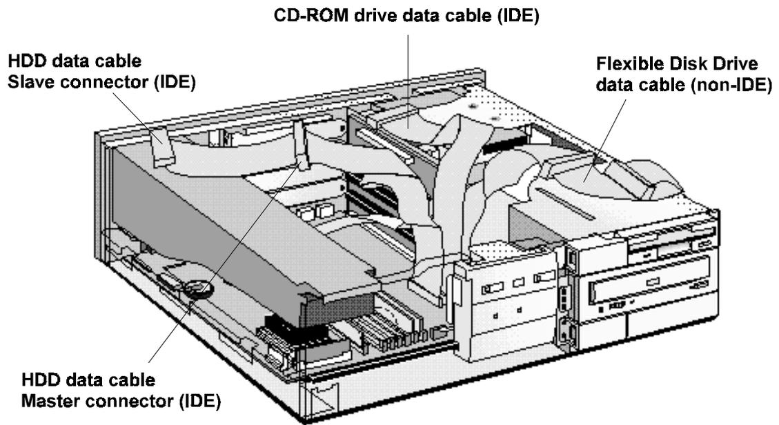
Up to three IDE devices can be connected to the system board using these data cables. (Refer to the storage device's manual to check whether you need to set jumpers, or if there are any special installation procedures.)
