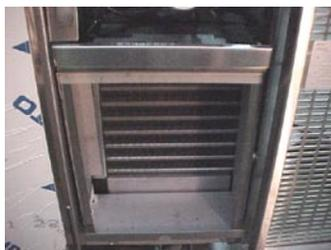
**Step 7:** Removing the filter also allows access to the condenser for cleaning.
