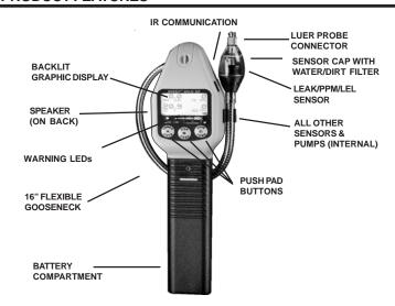
**Sensit**®**Gold G2** instruments are constructed of durable high impact ABS plastic to withstand the rigors of field use.
