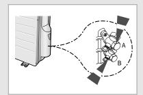
You must check if there is a gas leak before completing all the installation process. (connecting the assembly pipe and hose between indoor unit and outdoor unit, insulating the cables, hose and pipe, and fixing the indoor unit to the installation plate)
