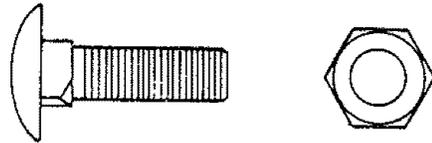
14. Secure L.H. baffle and R.H. baffle to mower housing using: four clamps, four 1/4 hex bolts and four 1/4 locknuts (shown full size below). Clamps and hardware furnished with grass catcher.
