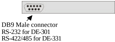
Figure 1-3. NPort Server Lite–Back Panel (DE-301/331)
