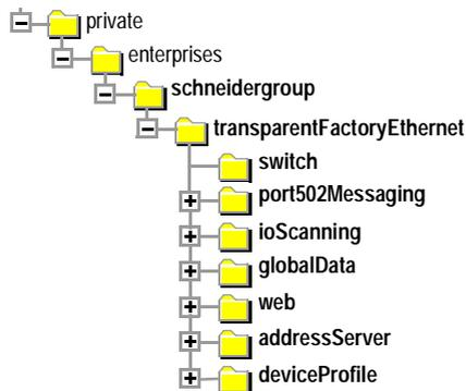
The source file of the **Ethernet Transparent Factory MIB** is available on the TSX ETG 1000 module. It can be downloaded from an Internet browser by clicking the **MIB Upload** link on the **Diagnostics** (See *Home Page*, p. 59) home page. The MIB version is 1.2. This file can be compiled with most commercial SNMP Managers.
