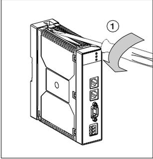
A line drawing of a module in its support plate. A screwdriver is shown from the right, with its tip under a screw on the top edge of the module. A curved arrow indicates the counter-clockwise rotation to loosen the screw. A circled number '1' is placed near the screwdriver's handle. |
