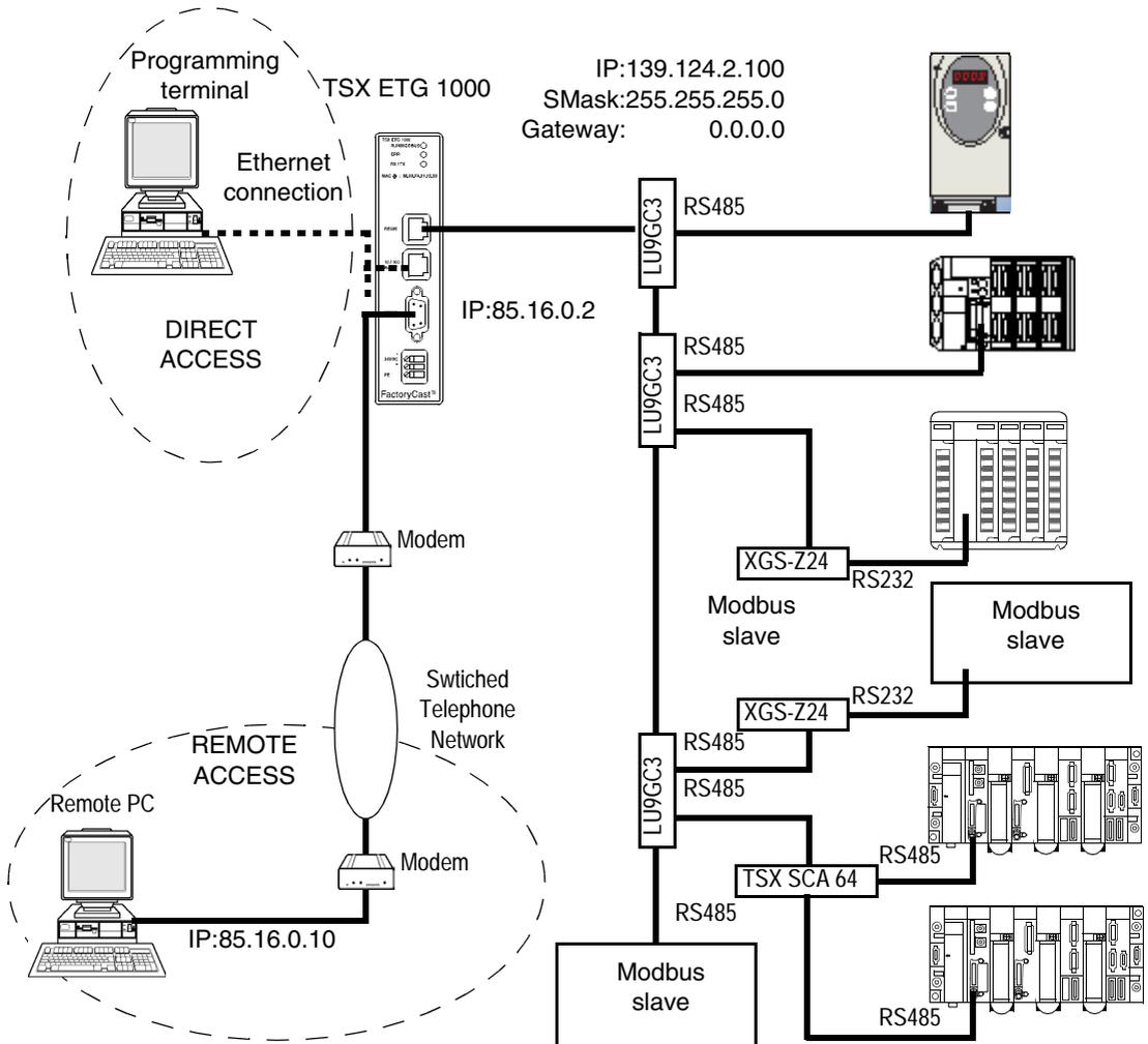
**Note:** To connect LU9GC3 to a TSX ETG 1000, you must use cable reference **VW3A8606R30** (RJ45-RJ45 cable).
