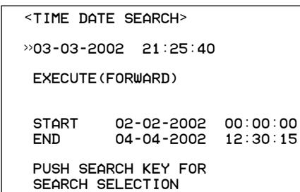
>To exit the <TIME DATE SEARCH> screen without searching, turn the SHUTTLE ring counterclockwise or press the *SEARCH* button twice.
