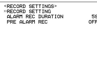
3. Check to see that the cursor is positioned at "RECORD SETTING", and then turn the SHUTTLE ring clockwise.
