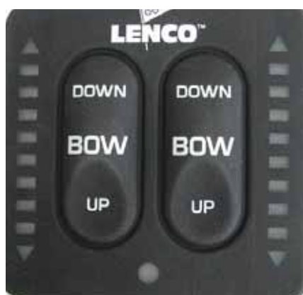
Trim Tab Switches
