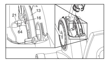
Slide the Reed Switch (21) slightly closer to or away from the Pulley Magnet (16), and then retighten the M4 x 16mm Screw (64). Turn the Pulley (13) for a moment. Repeat these actions until the console displays correct feedback.
