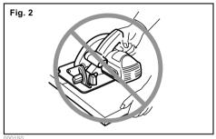
Never attempt to saw with the circular saw held upside down in a vise. This is extremely dangerous and can lead to serious accidents.
