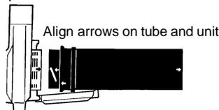
4. To attach the lower vacuum tube to the upper vacuum tube, first align the arrows on the two tubes. Then, press the two tubes together until the lower tube is securely seated in the upper tube (about 3 inches).
