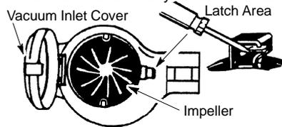
3. Turn the inlet restrictor counterclockwise and remove it from the unit. Do not close the inlet door. You will next attach the vacuum tubes.
