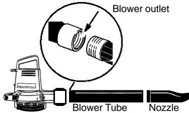
For Model 2695 only, the blower extension tube and nozzle are combined into one component.
