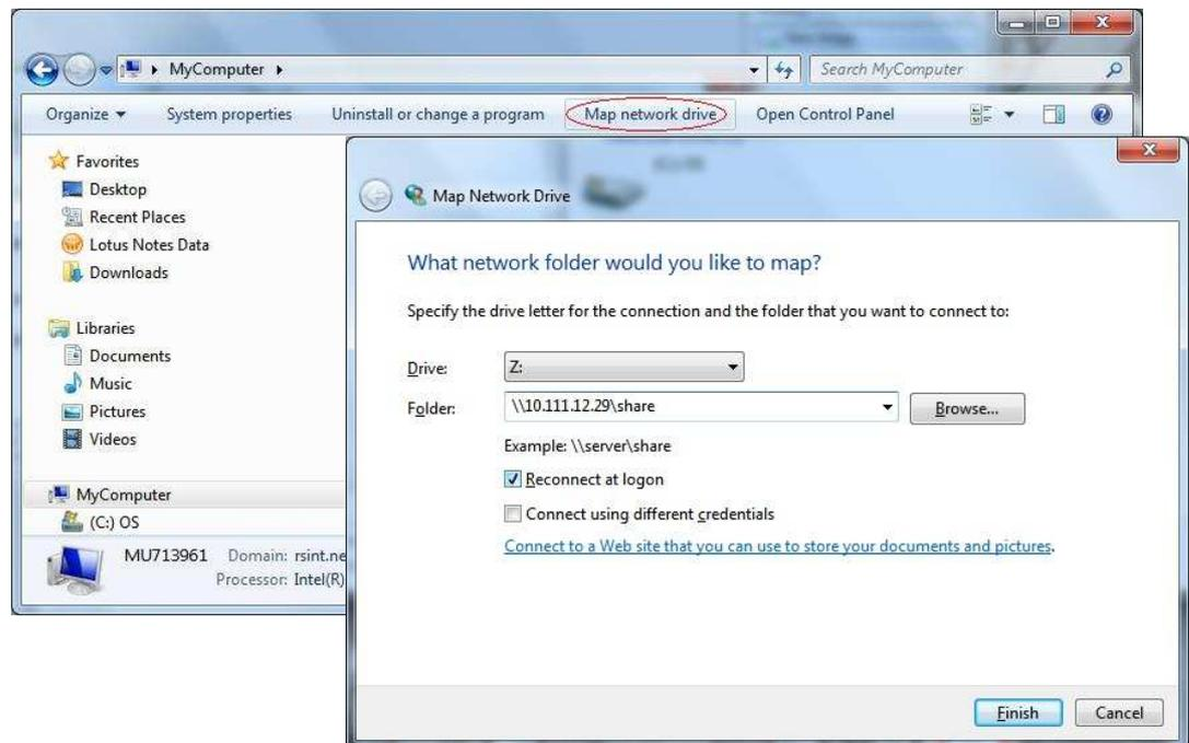
**Fig. 35: Map a network drive to an SMB/SAMBA folder**
