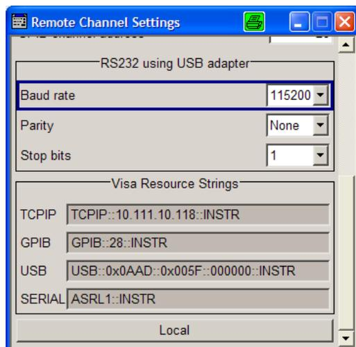
**Fig. 13: Setting up the serial interface**
