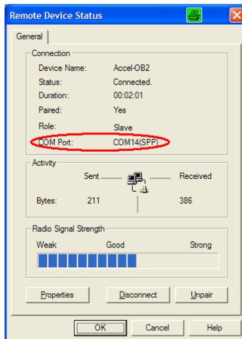
**Fig. 17: Detecting the active COM port**
