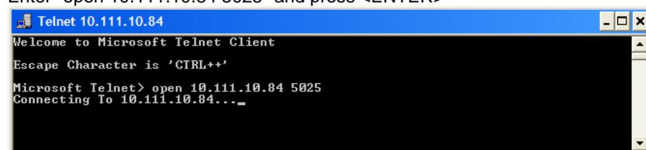
*Fig. 10: Telnet – connecting to signal generator*
