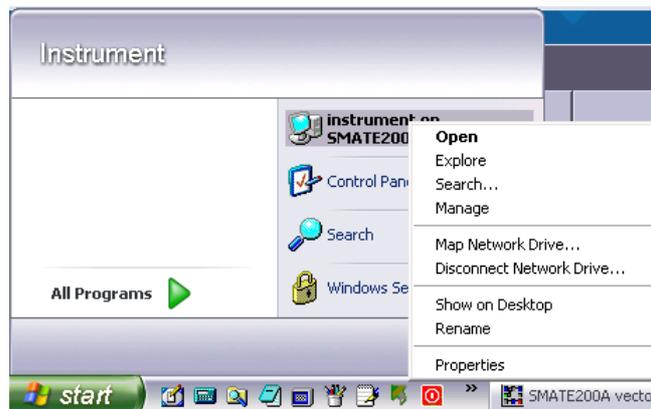
Fig. 21: Enabling remote desktop access (step 1)
