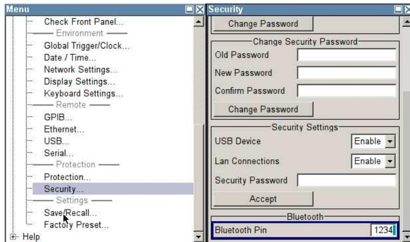
**Fig. 14: Input of the Bluetooth pin**
