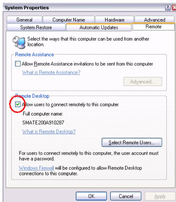
Fig. 22: Enabling remote desktop access (step 2)
