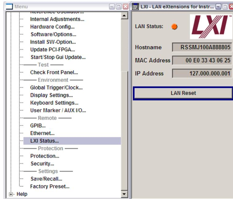
**Fig. 2: Finding the hostname and IP address on Windows instruments**
