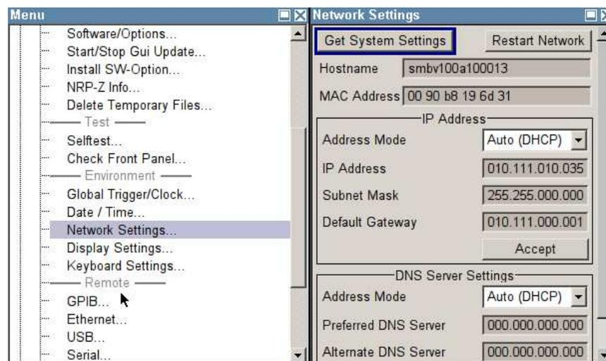
**Fig. 3: Finding the hostname and IP address on Linux instruments**
