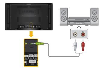
Connect a set of audio cables between the AUX L, R jacks on the AUDIO SYSTEM and [AUDIO OUT] on LCD Display.
