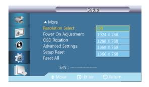
When the picture is not displayed properly on the screen when setting the graphics card resolution of the computer to  $1024 \times 768 \ @ 60$ Hz,  $1280 \times 768 \ @ 60$ Hz,  $1360 \times 768 \ @ 60$ Hz or  $1366 \times 768 \ @ 60$ Hz, by using this function(Resolution Select), you can have the picture displayed on the screen in the specified resolution.
