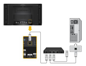
1. Connect the LAN cable between the [LAN] port on the product and the [LAN] port on your PC.
