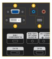
6 RGB/COMPONENT IN (PC/COMPONENT Connection Terminal (Input))
