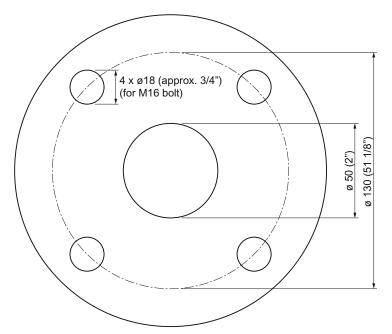
Figure 12-2 Dimensional drawing customer flange DN50/PN10-40, all measures in mm (inches)
