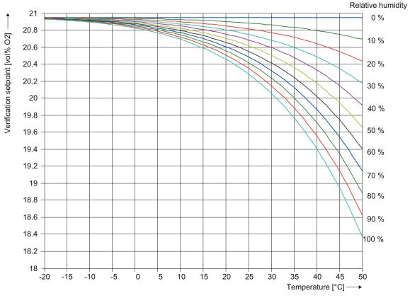
Figure 9-2 Verification set point for different relative humidities and temperatures.
