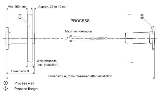
Figure 4-3 Flange alignment
