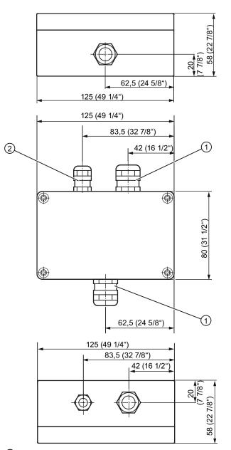
① Cable gland for sensor connection cable, M20 with plug
