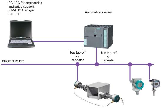
Figure 3-2 Example of a system configuration with PROFIBUS DP
