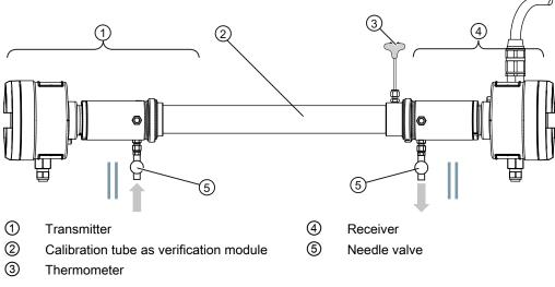
Figure 13-1 Calibration setup of SITRANS SL for oxygen applications
