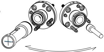
If this is done correctly the sensor pair is now aligned and should stay so even when the sensor bodies are removed and put back again. The system is designed to stay aligned even if a new receiver/transmitter unit is installed as replacement of an existing one.
