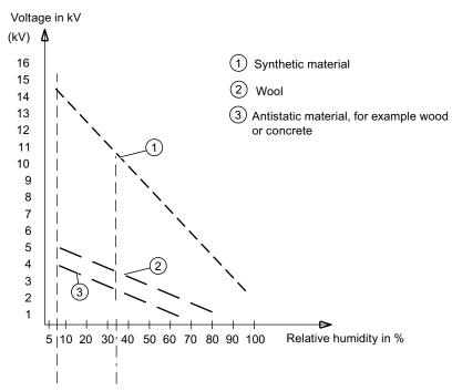
Figure A-2 Electrostatic voltages that can be charged to an operator
