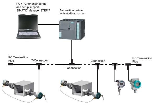
Figure 3-3 Example of a system configuration with modbus
