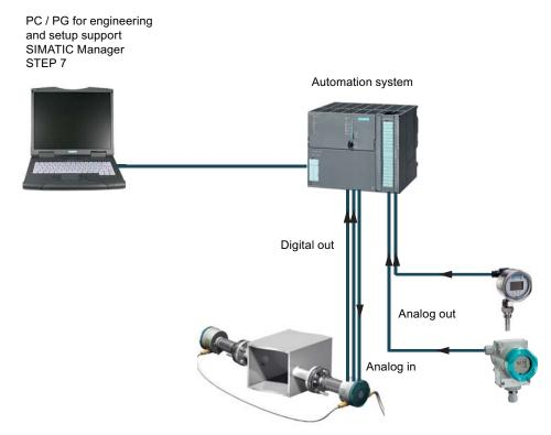
Figure 3-1 Example of a system configuration with analog I/O and digital I/O
