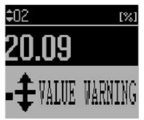
Figure 2-4 Local user interface (LUI) of SITRANS SL in the receiver unit (display of measured value)
