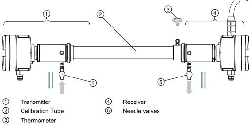
Figure 9-1 Verification tube setup
