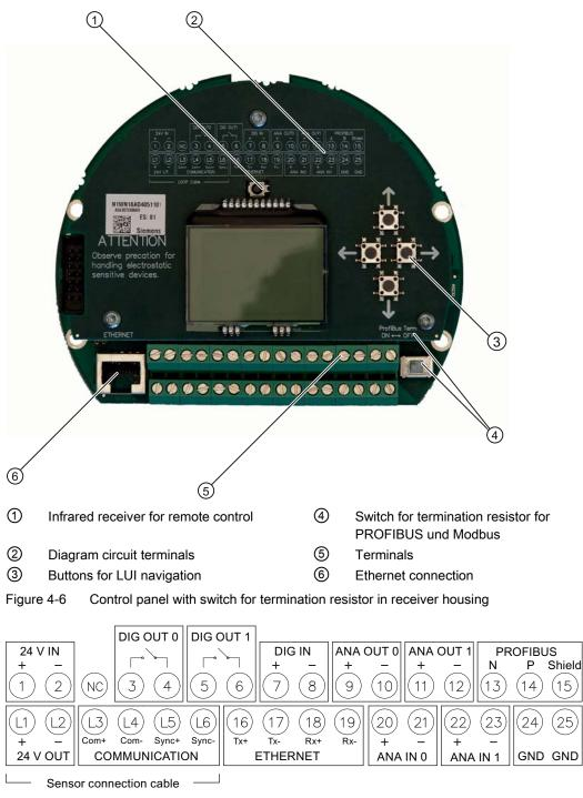
Figure 4-7 Diagram circuit terminals
