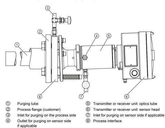
Figure 2-9 Arrangement for purging on the sensor side of the SITRANS SL
