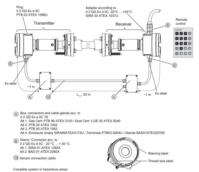
The figure below shows the cabling of the transmitter and receiver sensors.
