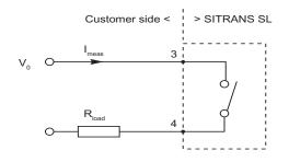
Figure 5-14 Using digital output
