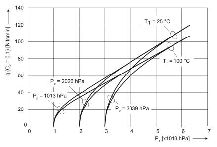
Figure A-1 Purge air flow rate
