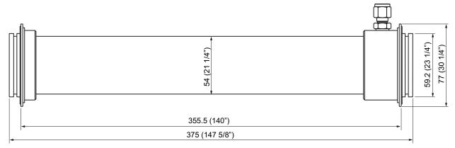
Figure 12-4 Dimensional drawing calibration tube, all measures in mm (inches)
