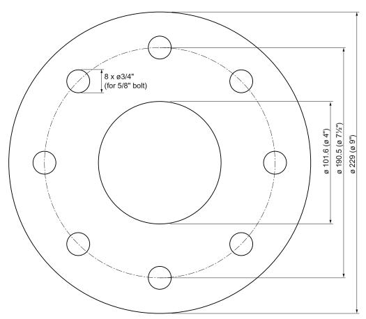
Figure 12-3 Dimensional drawing customer flange ANSI 4"/150 lb, all measures in mm (inches)
