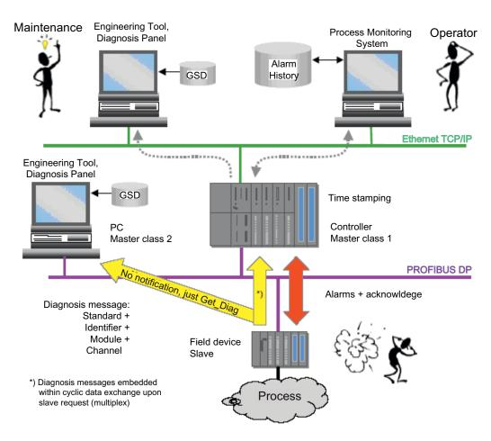
Figure 10-4 Diagnosis and alarm handling in PROFIBUS DP
