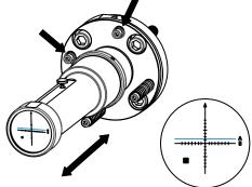
12. Align the transmitter using the supplied Allen key until the focused spot appears in the center of the crosshair corresponding to your SITRANS SL variant in the following table:
