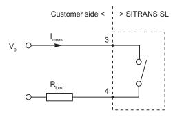
Figure 5-6 Using digital output
