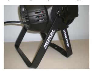
Clamp Mounting: The MICROH LED MAX ZOOM TRI provides a unique mounting bracket assembly that integrates 2 brackets to be used to mount on a truss or the floor. When mounting this fixture to truss, be sure to secure an appropriately rated clamp to the included bracket fitted through the center hole. As an added safety measure, be sure to attach at least one properly rated safety cable to the fixture.
