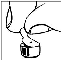
Before inserting a new battery in your hearing aid, remember to remove the adhesive tab. Do not use batteries on which there is a sticky residue from the tab or other unwanted substance as this can block the battery airholes.
