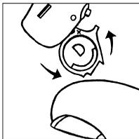
The battery must be placed with the plus (+) sign visible, in accordance with the plus (+) sign on the battery drawer. If the battery drawer does not close easily, the battery is incorrectly inserted.
