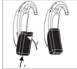
Slide the audio shoe onto the hearing aid, as shown. Press the shoe gently onto the aid until you feel a click.
