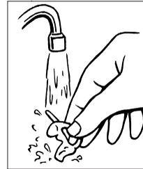
If this is not sufficient, disconnect the plastic tube from the hook of the hearing aid and wash the earmould in luke-warm water and a mild dish-washing soap. Rinse in cold water. Allow the earmould to dry overnight.
