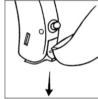
The battery drawer also functions as the on/off switch. The hearing aid is turned on when the switch is pushed upwards, and off when the switch is pushed downwards as illustrated.
