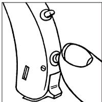
**Switch to “T”:** Your hearing aid is equipped with a telecoil. You can activate it by pressing the button briefly *once* (for approximately 1 second). Bravo will signal the change by making *one* brief beep-tone.
