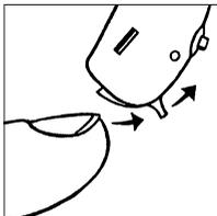
The battery drawer swings out on the opposite side of the on/off switch.
