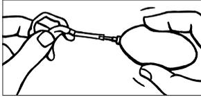
If there is still moisture in the earmould or tube, use a syringe or a small blower to blow it dry. Do not use alcohol to clean your earmould!
