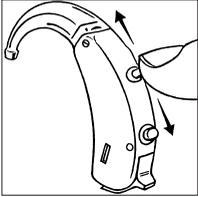
Your hearing aid has a digital volume control, shaped like a small lever. Push the lever upwards to raise the volume. Push the lever downwards to lower the volume. Use short touches for minor corrections of the volume.
