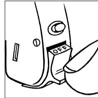
The word “OFF” is clearly visible on the switch when the hearing aid is turned off.
