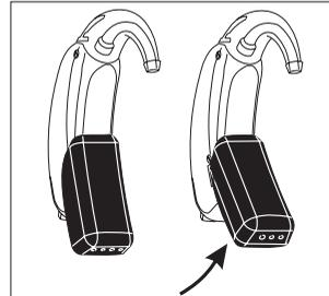
Remove the audio shoe by gently sliding it off and pulling it away from the hearing aid, as shown.
