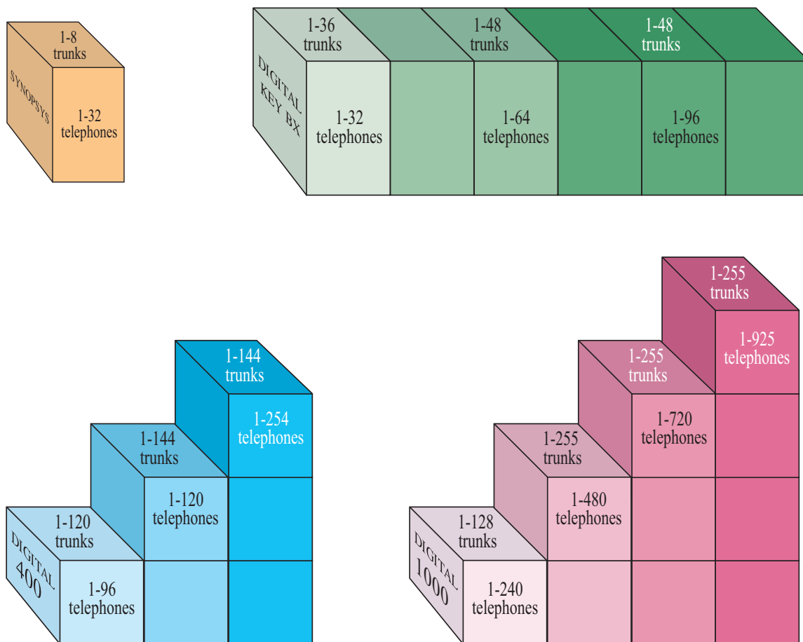
Figure 34 DIGITAL Family configuration capabilities
