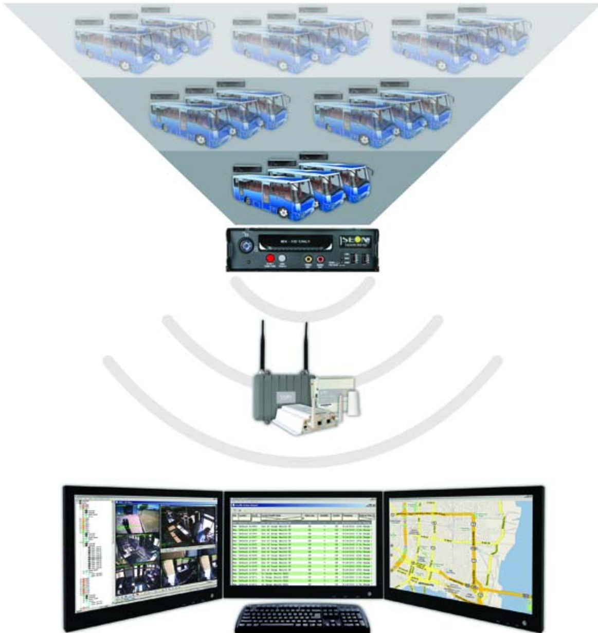
Figure 1-1 MX-HD DVR System with Smart-Reach Mobile Wireless and vMax Commander Software
