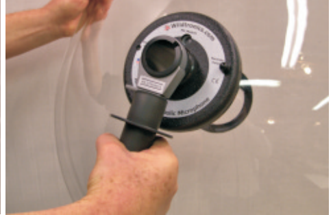
Tighten Handle clamp.
