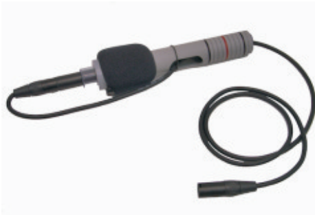
Inward facing mic in Mic Tube
