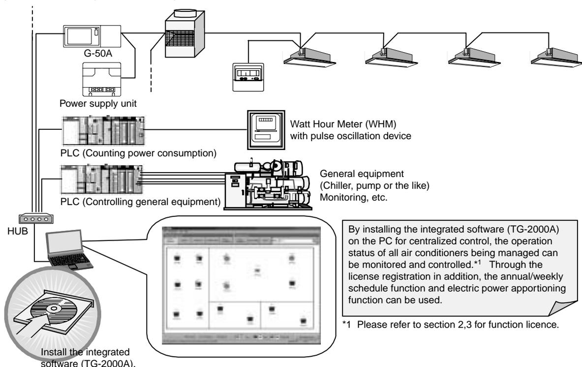
Figure 2-3 Outline diagram of integrated soft system composition
