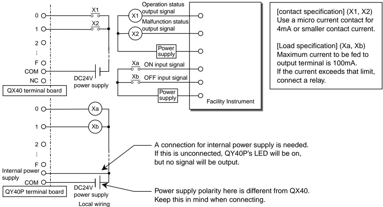
Figure 12-5 General-purpose control terminal connection diagram
