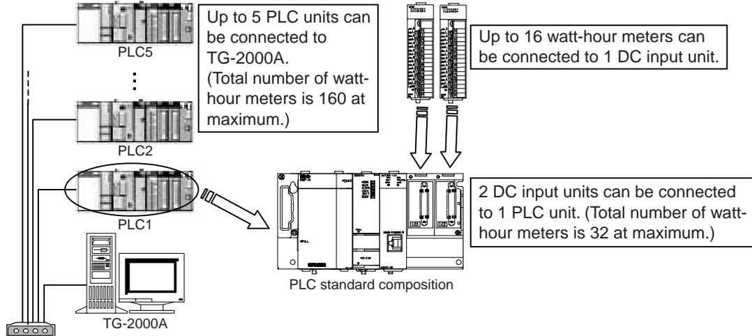
Figure 12-2 Restriction on the number of PLC units for the electric power apportioned charge function
