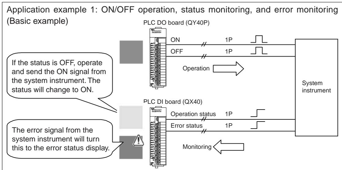
\*When the system instrument does not provide the output of operation status, connect to the input of operation status by installing a self-holding circuit.
