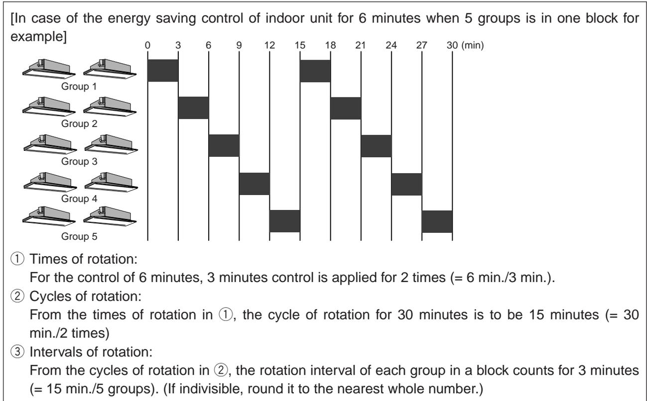
Figure 9-3 Example of indoor unit energy saving control
