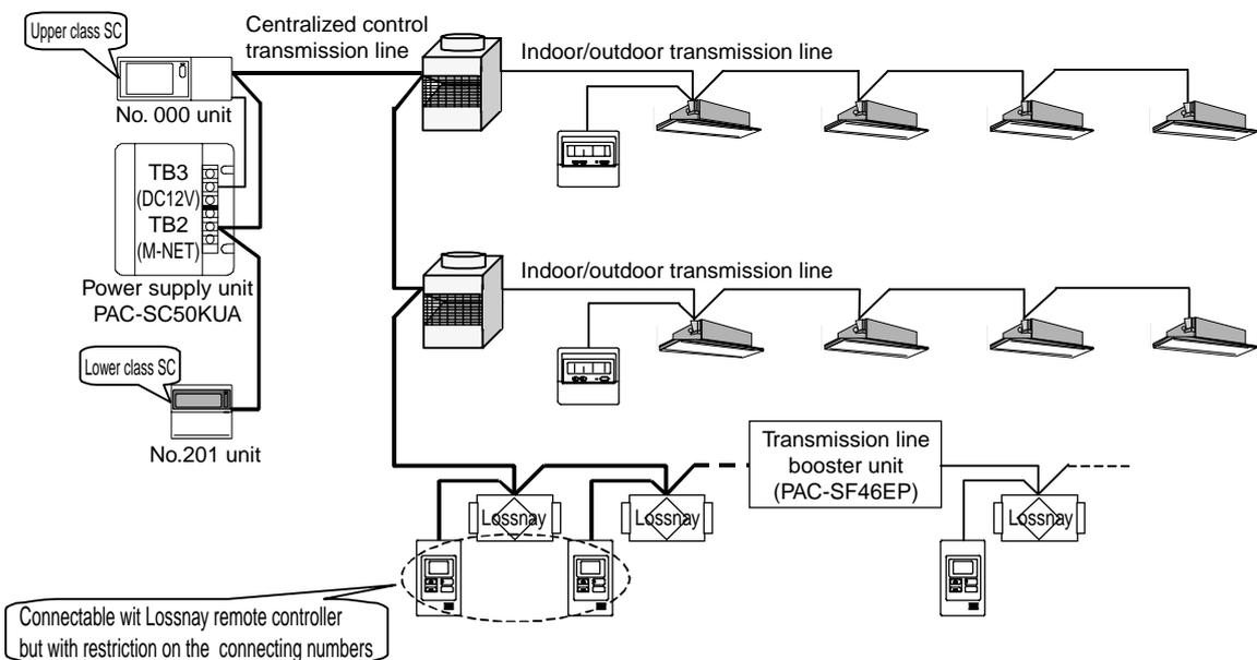
Figure 5-5 Connection of centralized control transmission line
