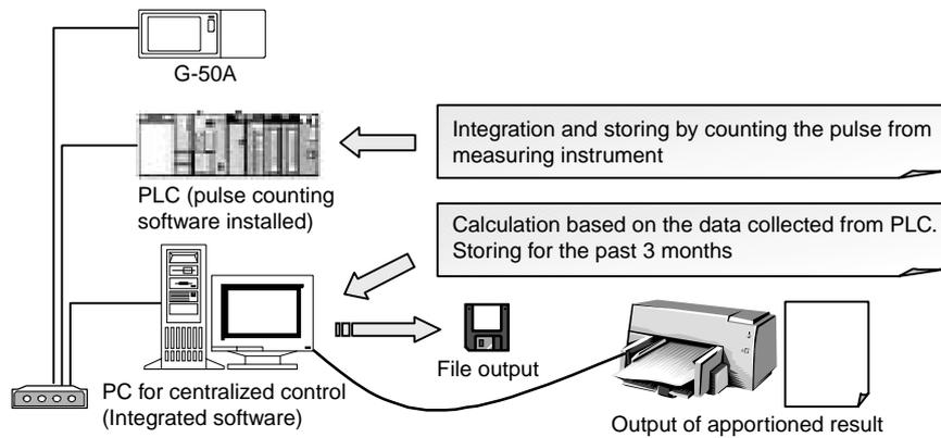
Figure 8-12 Mechanism of electric power pulse counting (direct reading) method
