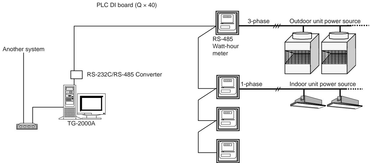
Figure 10-2 Outline wiring of measuring instruments
