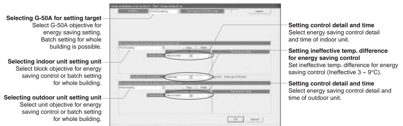
Figure 9-2 TG-2000A energy saving control setting screen
