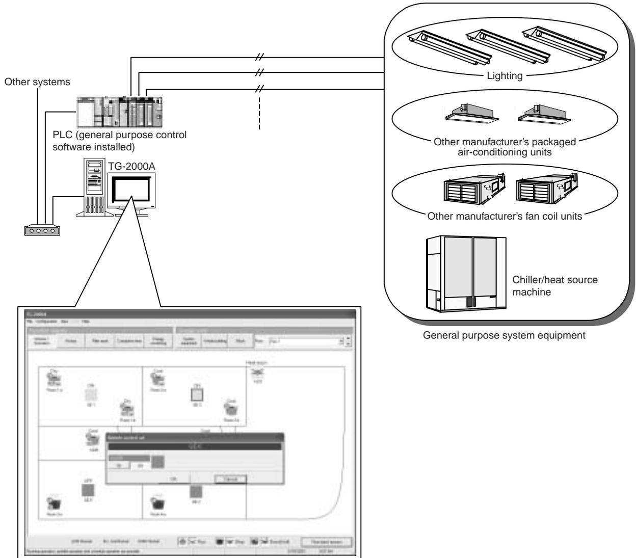
Figure 11-1 General purpose control system composition
