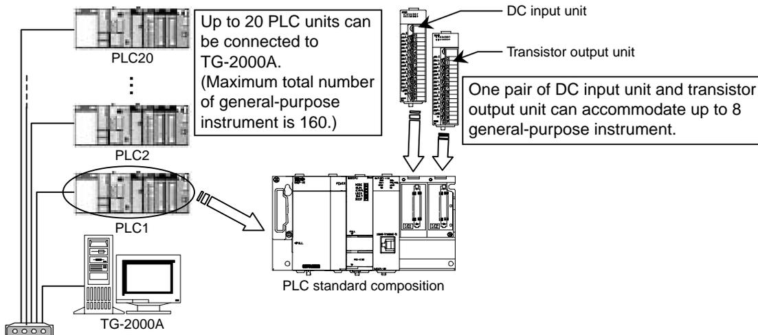
Figure 12-4 Restriction on the number of PLC units for multi-purpose control functions
