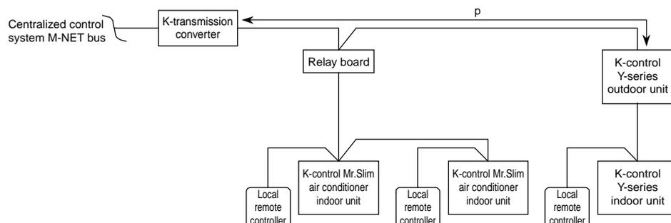
Figure 4-6 K-control mixing system example
