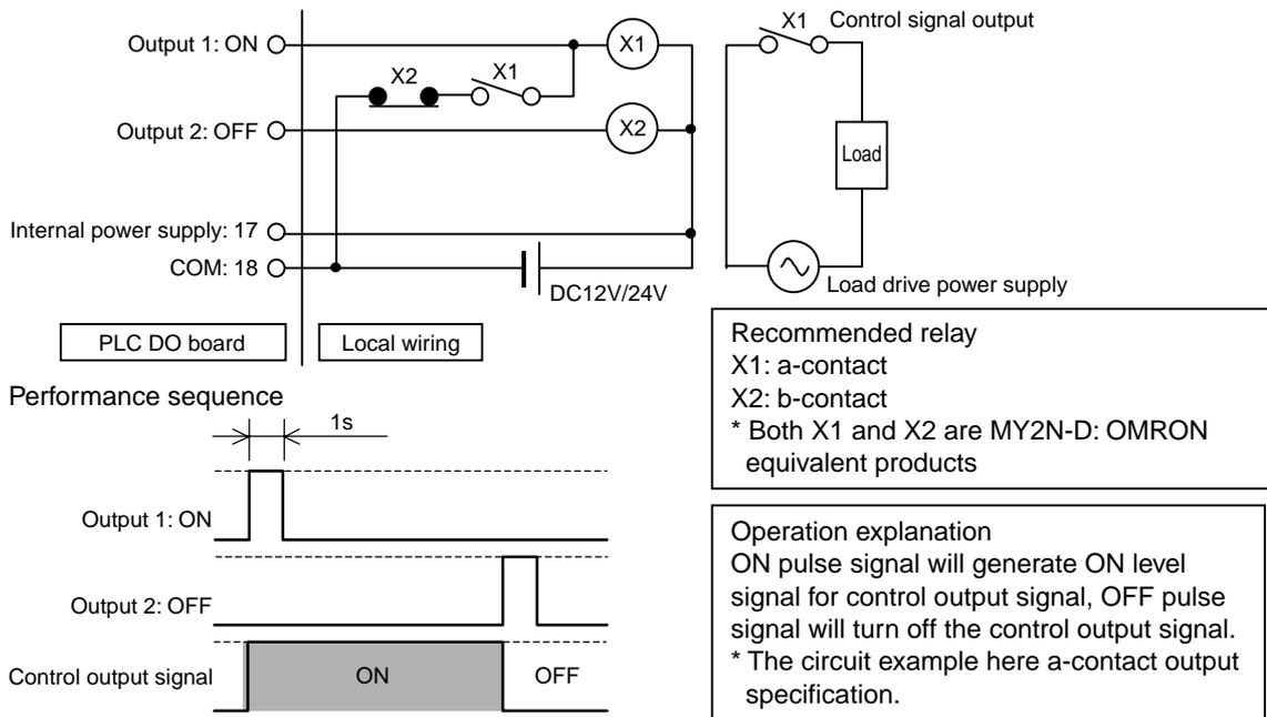
Figure 12-6 Pulse-level conversion circuit example
