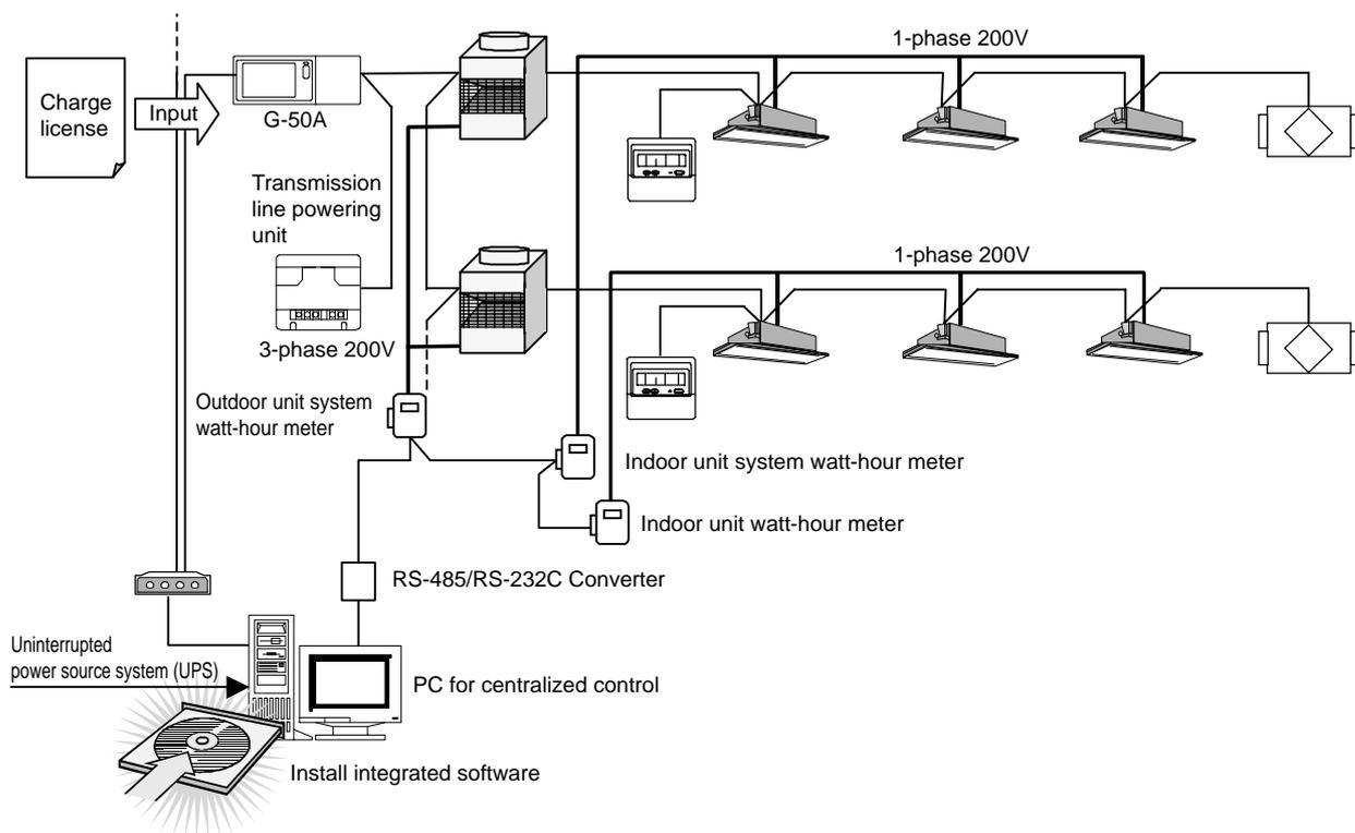
Figure O-O Basic configuration of power consumption PC direct reading system (RS-485 Watt-hour meter)
