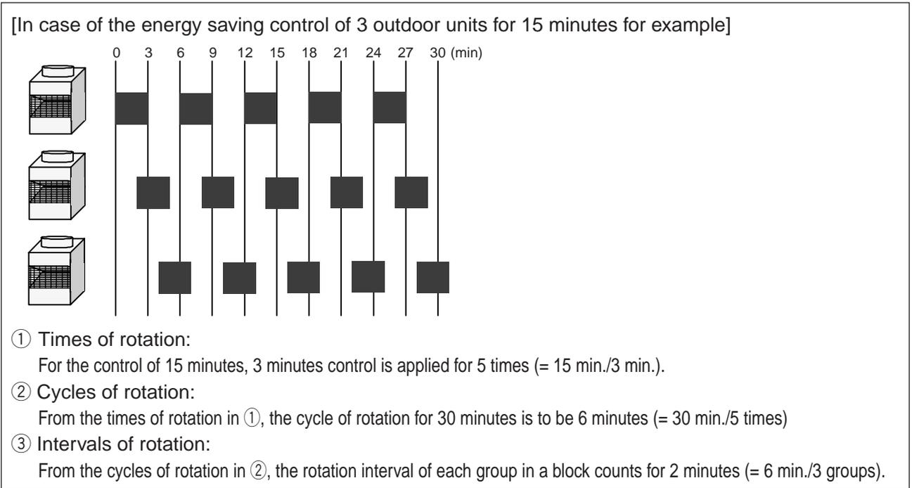
Figure 9-4 Example of outdoor unit energy saving control
