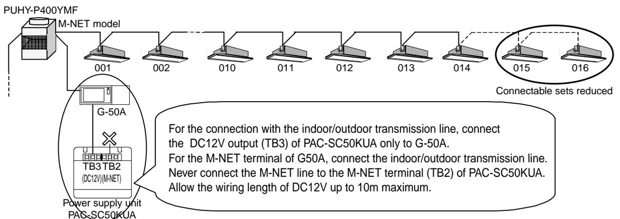
Figure 5-6 Connection of the indoor/outdoor transmission line
