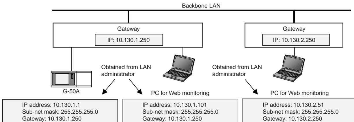
Figure 13-2 Setting example 1 of existing LAN system
