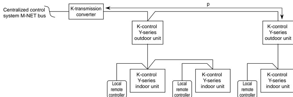
Figure 4-5 K-control Y-series wiring example
