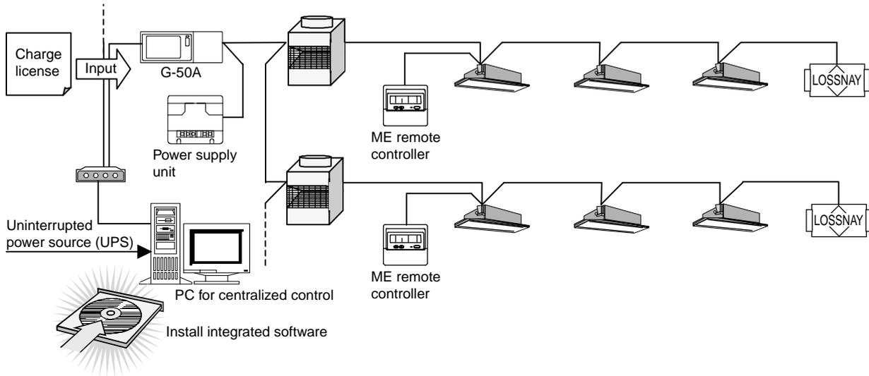
Figure 8-7 Basic composition of electric power manual input method
