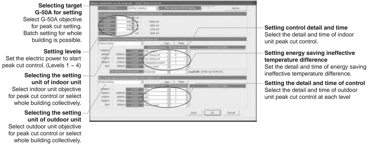
Figure 9-6 TG-2000A peak cut control setting screen
