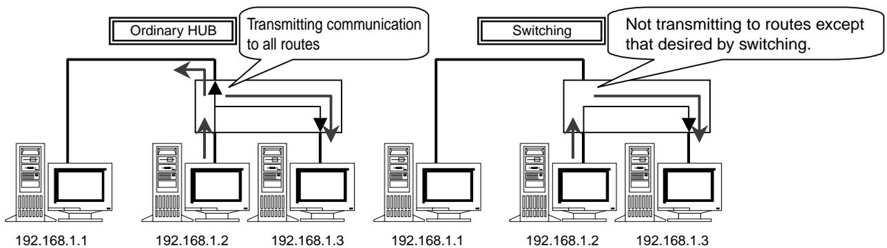
Figure 6-2 Switching hub concept
