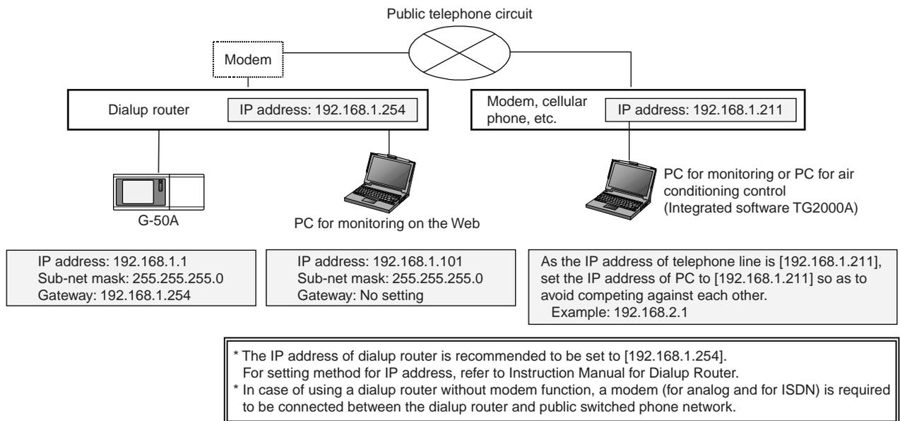
Figure 13-5 Setting example of remote monitoring system
