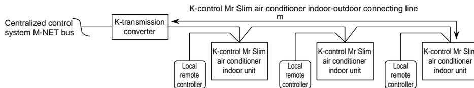
Figure 4-3 K-control Mr.Slim air conditioner wiring example
