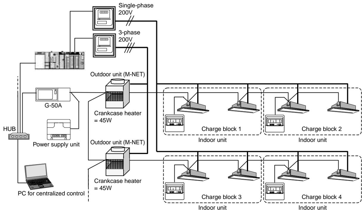
Figure 8-10 Example of charging system [Electric power pulse counting (apportioning) method]
