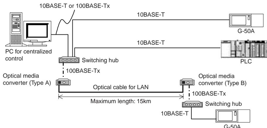
Figure 13-8 Chart of LAN system using optical cable
