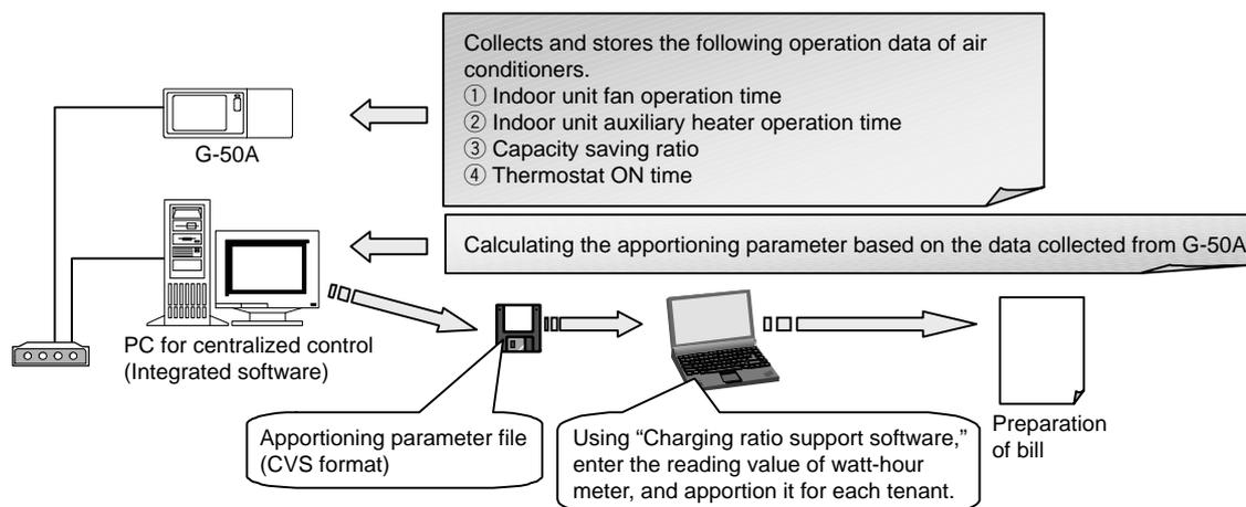
Figure 8-11 Mechanism of electric power manual input
