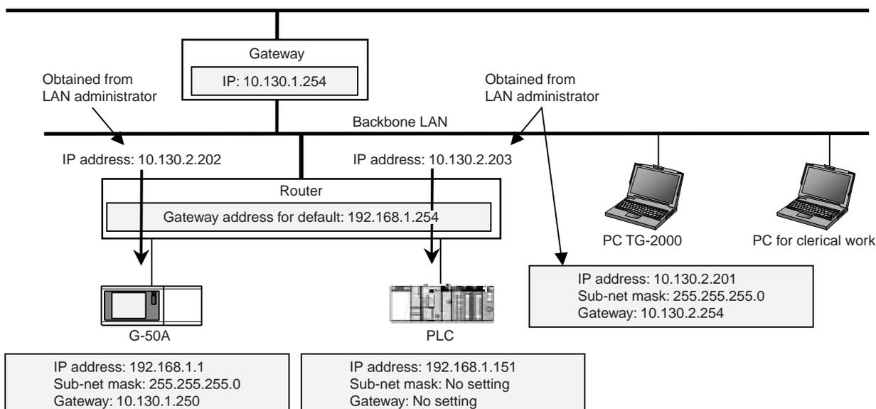
Figure 13-3 Setting example 2 of existing LAN system
