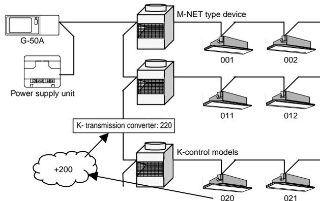
Figure 5-8 K-control converter address
