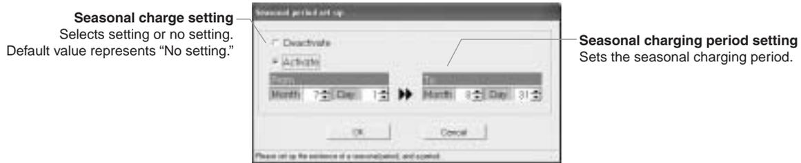
Figure 8-5 TG-2000A seasonal charge setting screen (ex, electric power manual input, pulse count)
