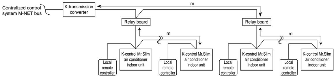
Figure 4-4 Relay board wiring example
