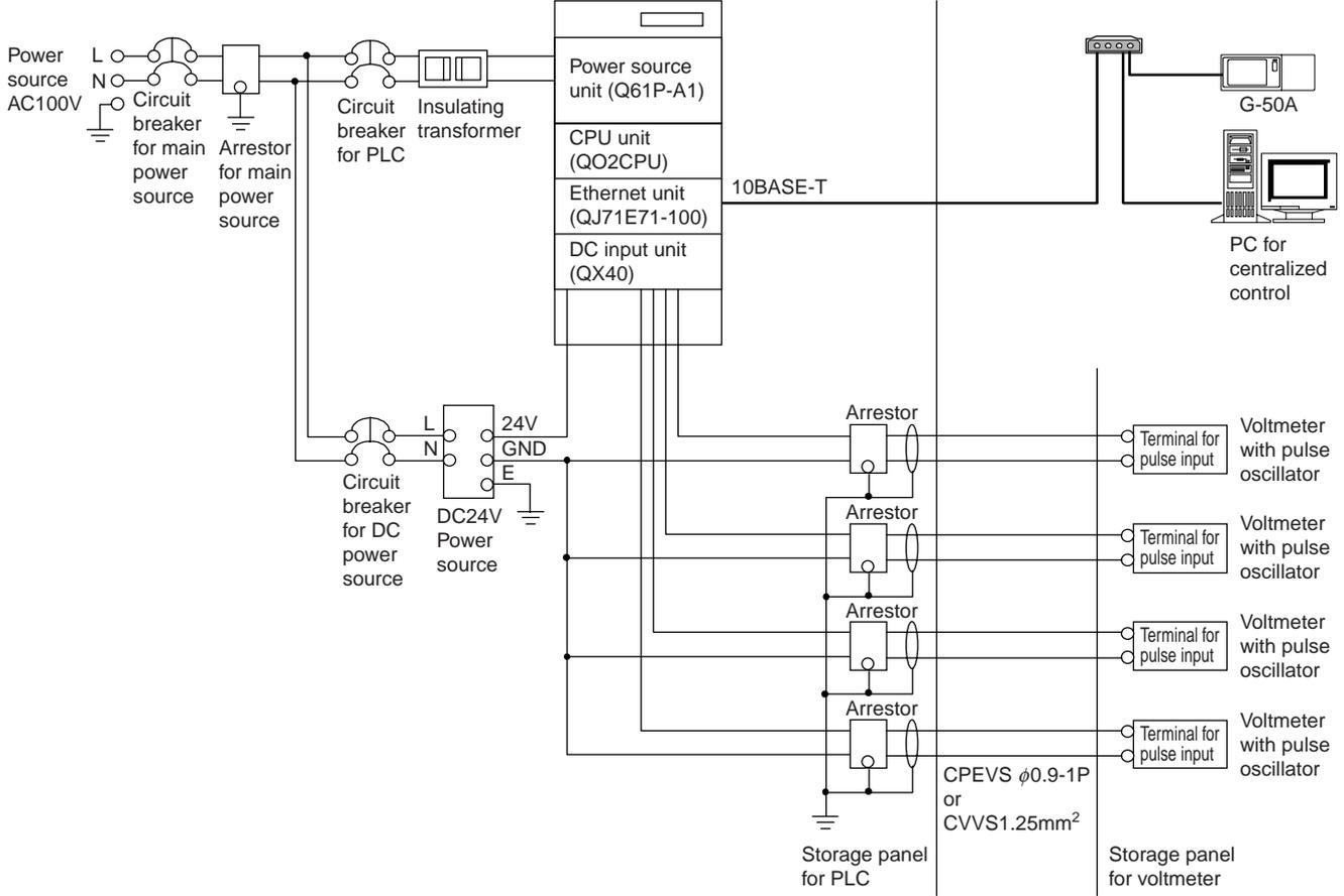
Figure 12-7 Wiring example around PLC
