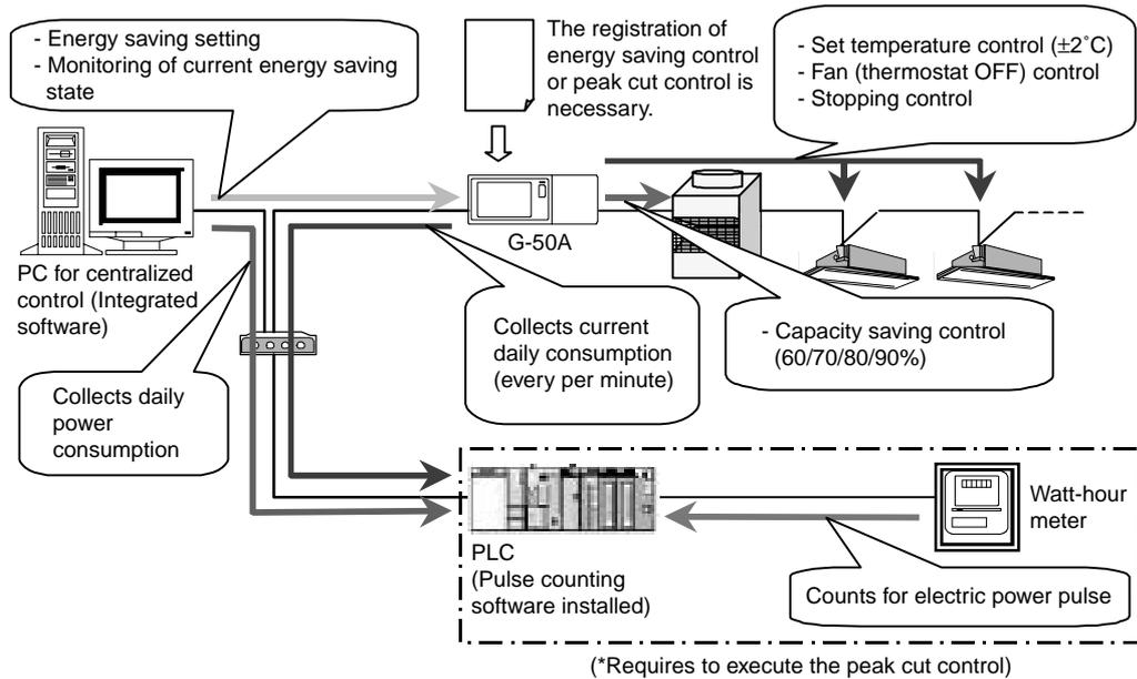
Figure 9-1 Energy saving/peak cut control system composition
