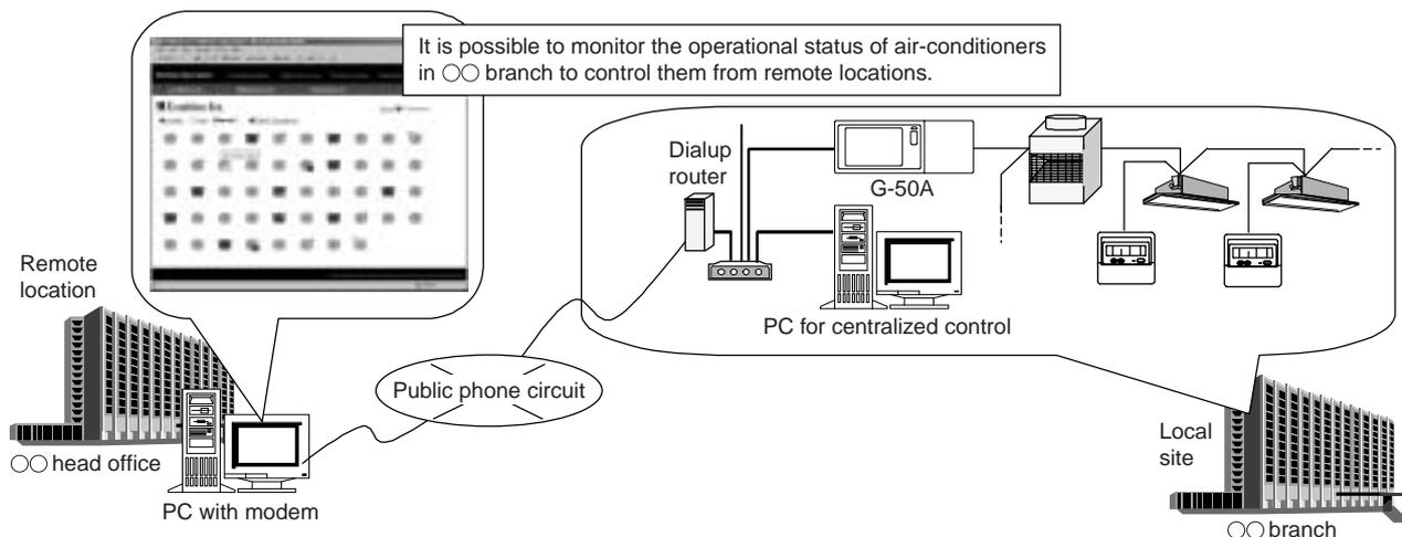
Figure 13-4 Remote monitoring system
