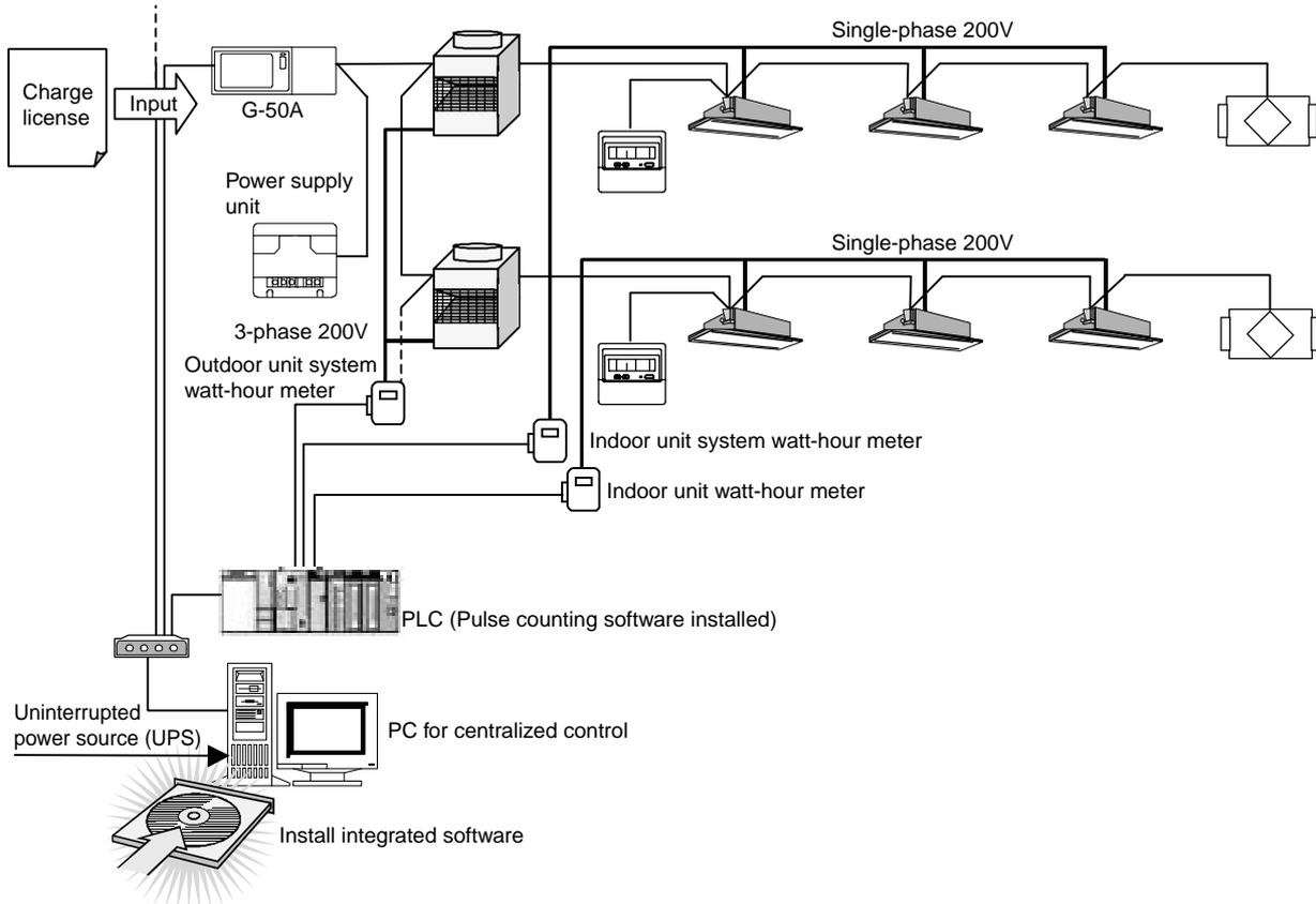
Figure 8-8 Basic composition of electric power pulse counting method
