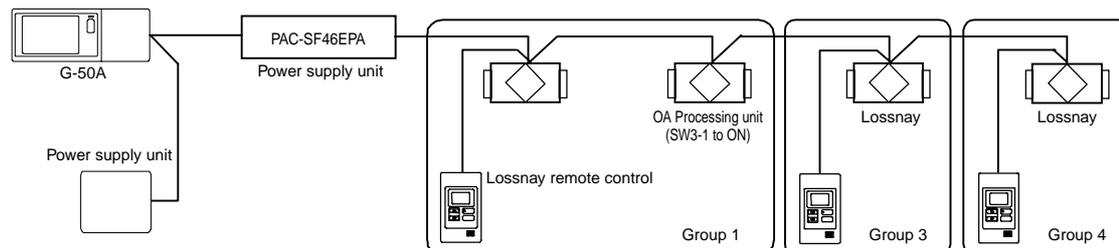
Figure 5-3 Electricity supply using a Lossnay system
