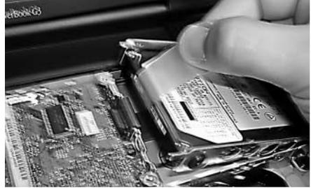
**Step 11:** Grasp the hard drive bracket by its sides and carefully pull the drive out of its compartment. You may have to gently but firmly jostle the drive from side to side to loosen it from its fasteners within the compartment.
