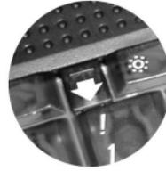
**Step 7:** Carefully rotate the keyboard so that it lays face down on the PowerBook's palm rest, being careful not to rip the ribbon cable attaching the keyboard to the logic board. Carefully disconnect the keyboard ribbon cable from the logic board.
