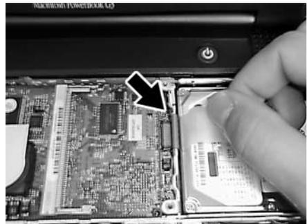
**Step 10:** Lift the plastic flap up to bring the end of the hard drive out of its compartment.
