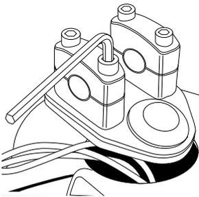
**1** Using the 6mm key wrench, remove bolts from handlebar clamp.
