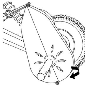
**3** Remove the 3 screws from the top half of the chain guard and remove.
