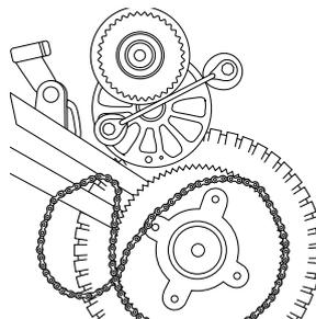
**6** Remove chain from both sprockets and replace with new chain.
