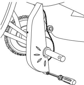
**4** Remove the 2 screws from the bottom half of the chain guard and remove.
