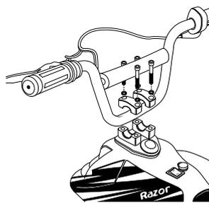
**2** Place handlebars in handlebar clamp in upright, vertical position.
