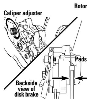
**3** If the brake rotor is dragging on the brake pads use your fingers to twist the caliper adjuster in either direction until rotor is centered between pads.
