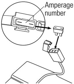
**4** Remove the fuse and replace with a new one of equal amperage.
