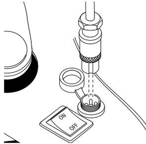
**1** Turn power **OFF** before charging. Align the groove on the plug of the charger port and plug into the port on the Dirt Quad.
