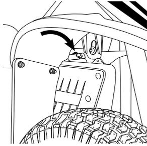
**2** Under the front fender and through the frame, locate the fuse box attached to the top of the battery.
