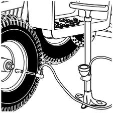
Using a bicycle-style tire pump equipped for a Schrader-type valve, inflate the tires to the PSI indicated on the sidewall of the tire.
