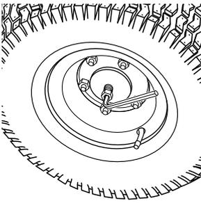
**1** Remove the bolt and washers on the outside of the rear wheel.
