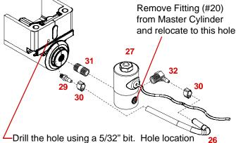
is .900" right of top left corner and .900" down from top of master cylinder. Tap hole with 10-32 NF tap
