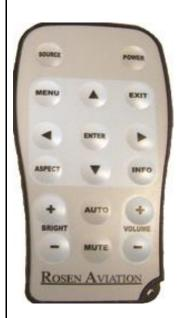
**Note:** The AUTO button works only when an RGB source is active. The MUTE and VOLUME ± buttons are not used.
