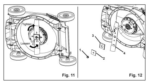
NOTE: Be sure to replace the parts in the exact order in which they were removed. When installing the cutting blade, verify that it is installed with the curved ends pointing toward the mower deck, and not toward the ground. Refer to the schematic drawing on page 31 of this Manual.
