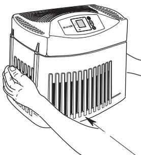
Align housing assembly bottom with top of base and reposition securely
