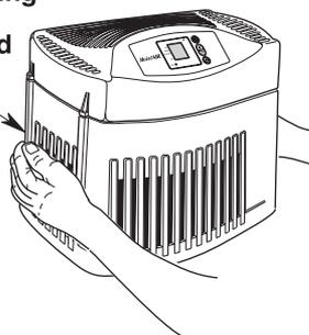
Position start and finish of coiled filter at centre of base
