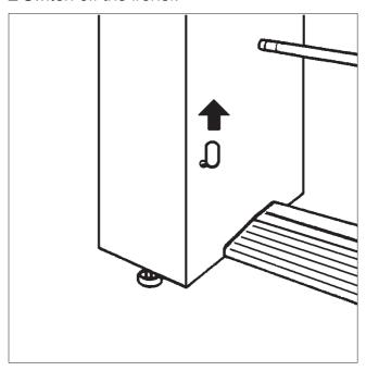
■ Lift the heater plate release mechanism upwards.
