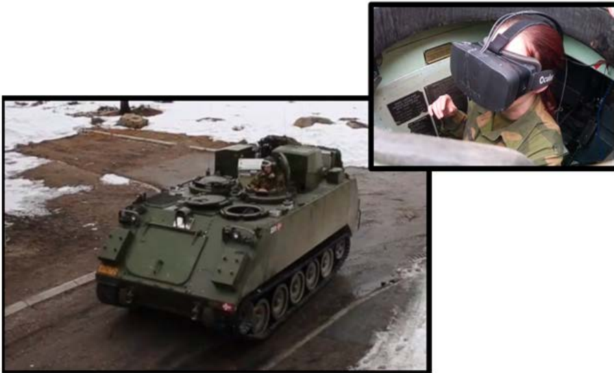
Figure 1.6: An experiment using the Rift to allow tank drivers to drive with the hatch closed as seen in a report on Norwegian TV station TuTV
