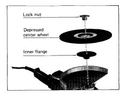
To tighten the lock nut, press the shaft lock firmly so that the spindle cannot revolve, then use the lock nut wrench and securely tighten clockwise.
