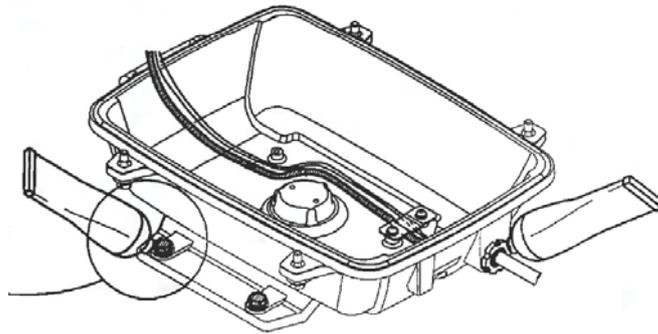
11. Use silicon sealant around the mounting bolts
