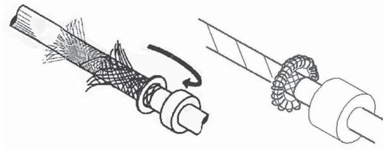
5. Pass the scanner cable through the cable gland opening, into the pedestal.
