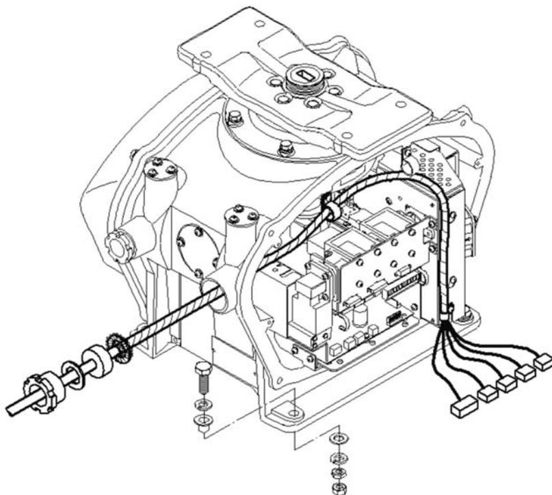
6. Connect the five scanner cable connectors to the 'J' connectors as follows:
