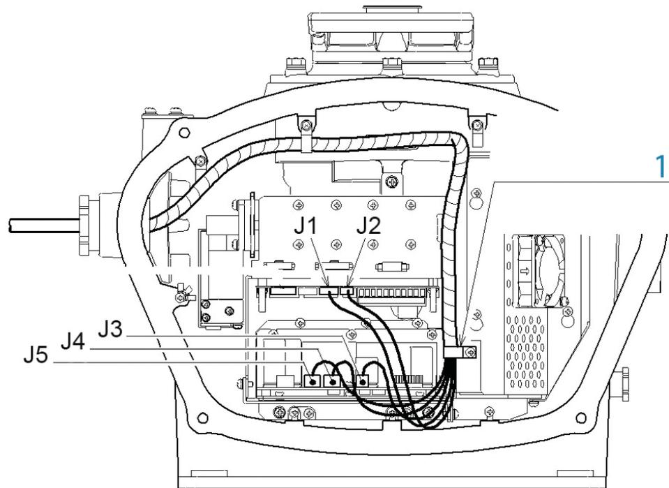
7. Use the cable clamp (1) to secure the cable to the upper housing. The clamp should hold the cable at the point where it is wrapped in copper tape.
