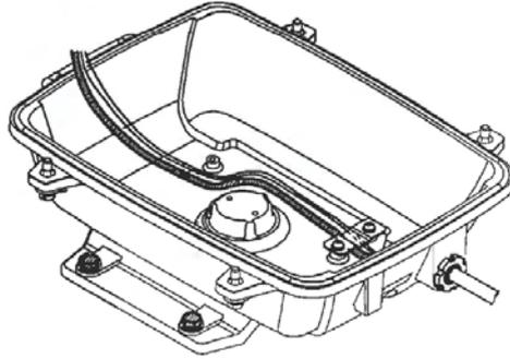
10. Fit the cable gland assembly. Use silicon sealant around the cable entry point.
