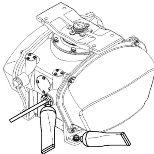
10. Use silicon sealant around the mounting bolts
