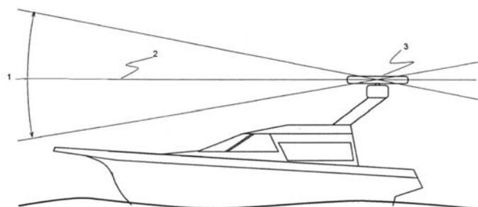
However, when a power boat is traveling at high speed, the bow rises up out of the water and if the elevation angle (trim) of the bow is raised up so that it equals, or exceeds, 50% of the vertical beam width of the radar, this can cause two problems:
