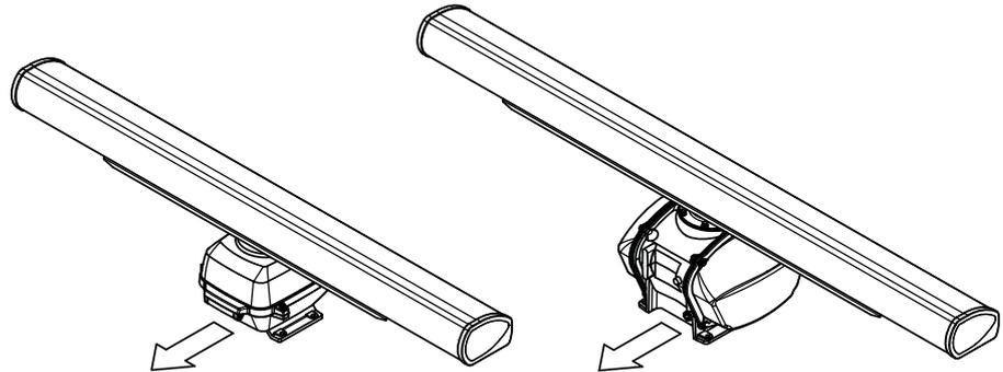
→ **Note:** In correct orientation, both the 10 kW and 25kW scanners have the scanner cable exiting towards the stern of vessel.
