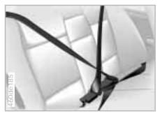
When transporting heavy cargo while the rear seat is unoccupied, secure each of the outside safety belts in the opposite lock (refer to the illustration).
