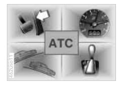
On vehicles with automatic transmission, the ATC (Adaptive Transmission Control) uses a number of factors to calculate the maximally efficient gear. In this process, it considers your individual driving style as well as current driving conditions.
