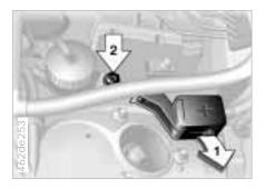
The cover of the positive terminal connector is marked with a "+" sign. Refer to the illustration. Remove by pulling the tab (arrow 1)
