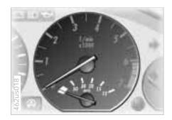
Indicates the current fuel consumption in mpg (on Canadian models in I/100 km). This instrument clearly shows whether your current driving style is conducive to economy and minimum exhaust emissions.
