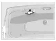
Bulbs in the luggage compartment lid: 1 Using a screwdriver, loosen the clip
