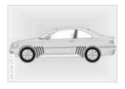
Near every wheel there is an antenna in the body that receives the signals from all four wheels. A central electronics system evaluates the quadruple signals and forwards any changes. The RDC plays an important part in driving safety.
