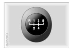
The shift lever's neutral plane (dot in the illustration) is located between 3rd and 4th gears.
