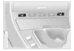
The seat cushion and backrest can be heated with ignition key in position 2.
