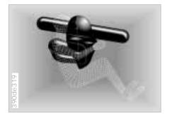
Deceleration sensors continuously monitor the physical forces acting upon the vehicle. If, as the result of a frontal collision, a deceleration is reached at which the protection of the safety belts alone is no longer adequate, the gas generators of the driver and passengerfront airbags are ignited. However, the passenger-side airbag is only triggered if an additional sensor has recognized that the passenger seat is occupied.
