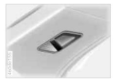
The reading lamps are located in the front near the interior lamp and in the rear of the vehicle (illustration). They can be switched on and off with the switch adjacent to each lamp.
