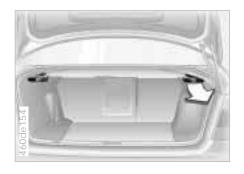
The rear backrest is divided into two sections, one-third and two-thirds of the seat respectively. For carrying longer objects, you can fold down either section of the backrest separately.
