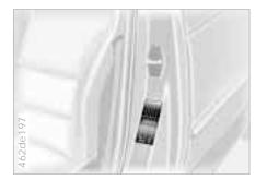
The inflation pressures are indicated on a sticker attached to the B-pillar behind the driver's door (visible with door open).
