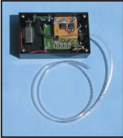
Photo 2 —Check out the completed water level sensor unit. The MC13192 SARD PCB, pressure sensor PCB, battery, and signal conditioning circuit are mounted in a standard black project box.
