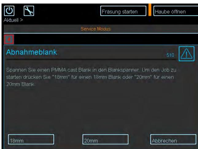
Clamp a PMMA cast blank into the blank clamp To start the job for a 18 mm blank select "18mm" or select "20mm" for a 20 mm blank.
