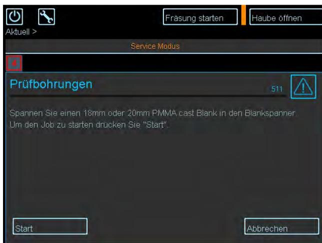
Clamp an 18mm or 20mm PMMA cast blank into the blank clamp. Press "Start" to start the job.
