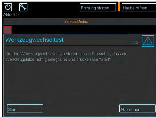
To start the tool replacement test, make sure that the tool slots are correctly occupied and then press "Start".
