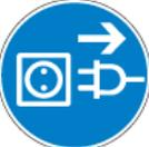
Disconnect the system from the power supply and the compressed-air feed before opening the stack:
