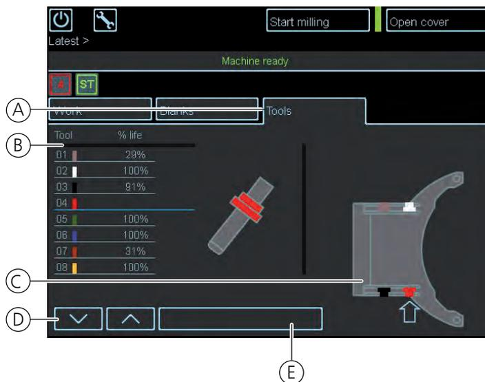
All information on tools and tool trays is contained in the "Tools" tab. You can see a list of tools and their remaining capacities. Exact information on colour coding of tools and their numbering is contained in Chapter " Colour coding of tools" auf Seite 72.
