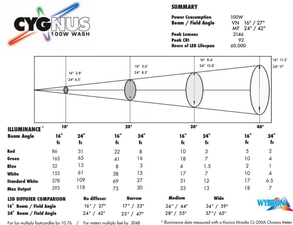
For lux multiply footcandles by 10.76 / For meters multiply feet by .3048
