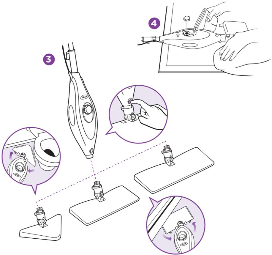
**3** Snap the mop head into the base to secure it. Press the release button to exchange mop heads.
