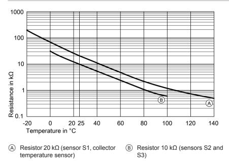
1. Disconnect the respective sensor and measure its resistance.
