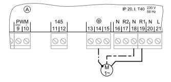
(A) Wiring chamber of the solar control unit
