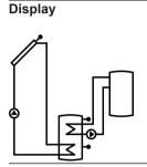
**Thermostat function** Output R2 is used for this function. Relay R2 switches subject to the temperature at S3 (see the following table).
