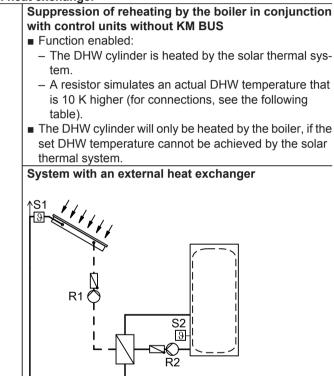
The secondary pump R2 is started in parallel with the solar circuit pump.
