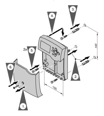
Before closing the solar control unit, make all electrical connections and apply a strain relief to all cables/leads. Installation sequence
