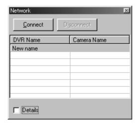
When you start the DX-PC25U, you see the Network box.. To view all the settings of the listed recorder or to register a new recorder, click the check box of Details.
