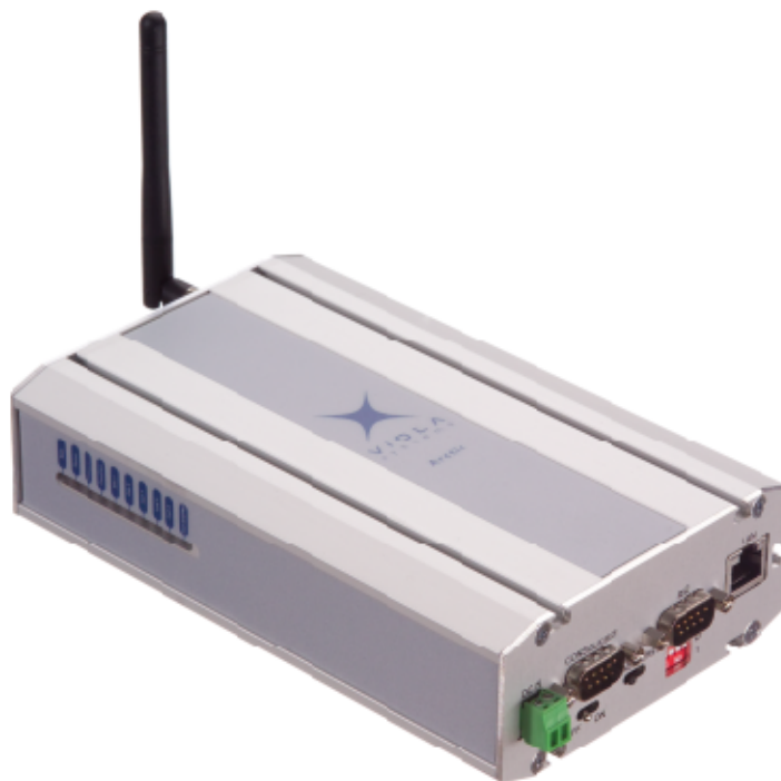
Figure 1. Arctic IEC-104 Gateway
