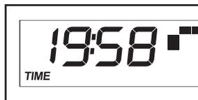
Note: When a resistance & rpm workout is selected, the display will show the time remaining in the workout instead of the elapsed time.
