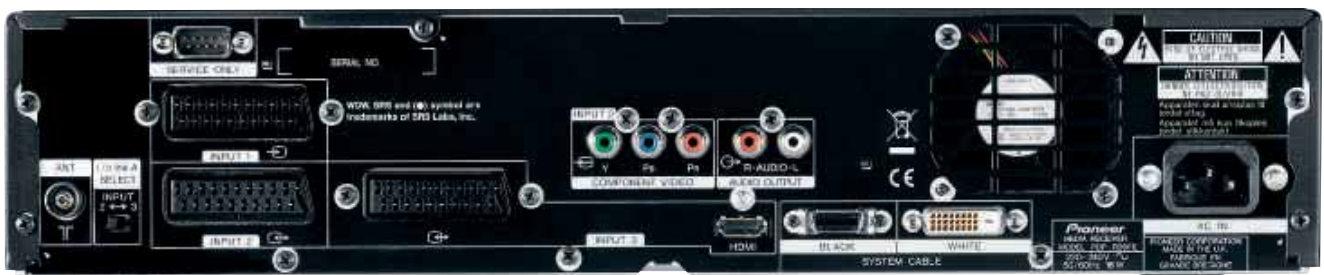
Rear Panel PDP-506FDE / PDP-436FDE
