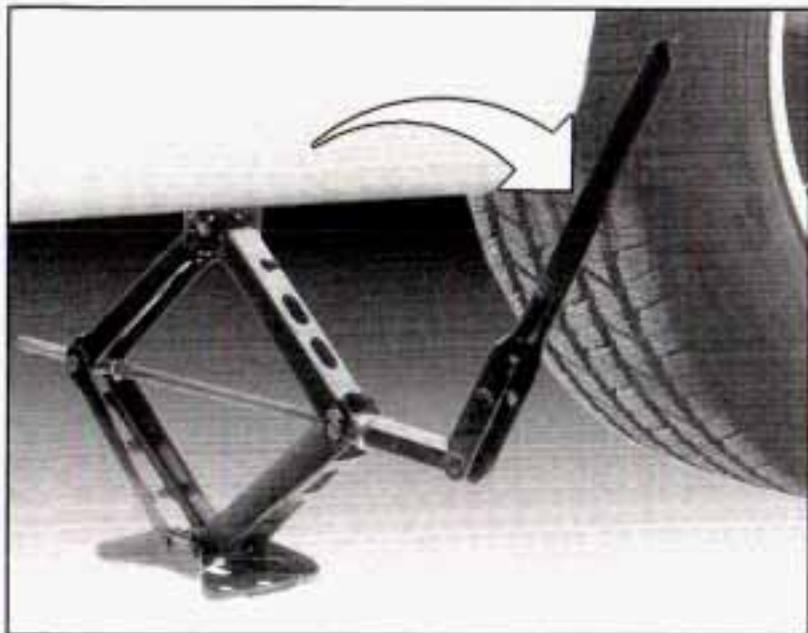
5. Raise the vehicle by turning the jack handle clockwise. Raise the vehicle far enough off the ground for the spare compact tire to fit underneath the wheel well.
