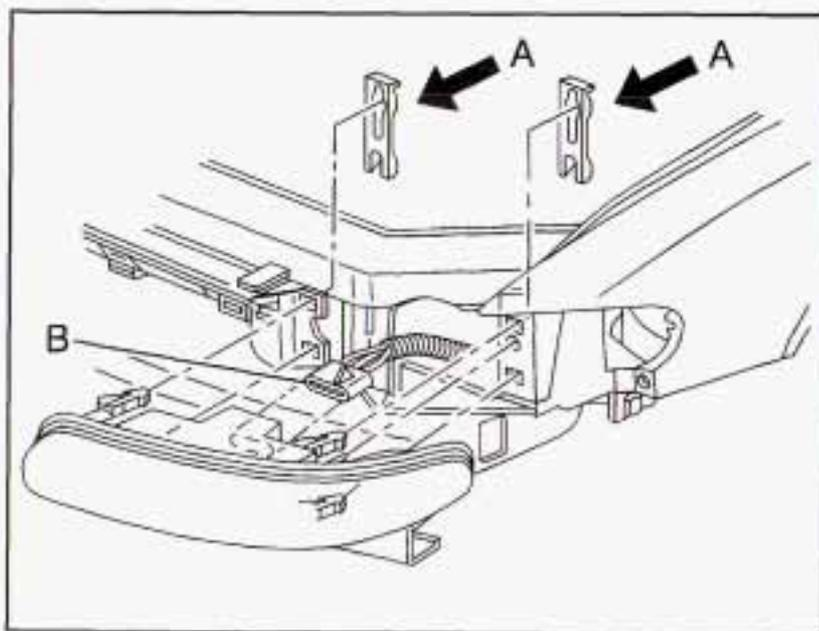
2. Pull up on the headlamp retainers (A) to release the assembly locator tabs.
