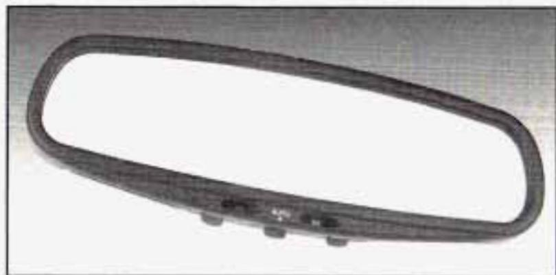
Your vehicle may have an automatic dimming rearview mirror. Push the button in the center of the mirror to turn this feature on. The mirror will darken gradually to reduce glare from headlamps behind you.
