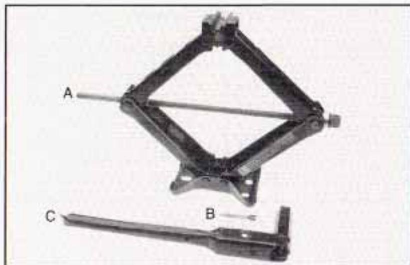
The tools you'll be using include the jack (A), extension and protection guide (B) and wheel wrench (C).
