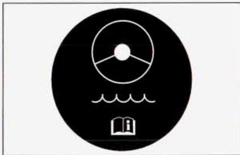
The power steering fluid reservoir is located on the passenger's side of the vehicle at the back of the engine compartment, and can be identified by the above graphic on the cap.
