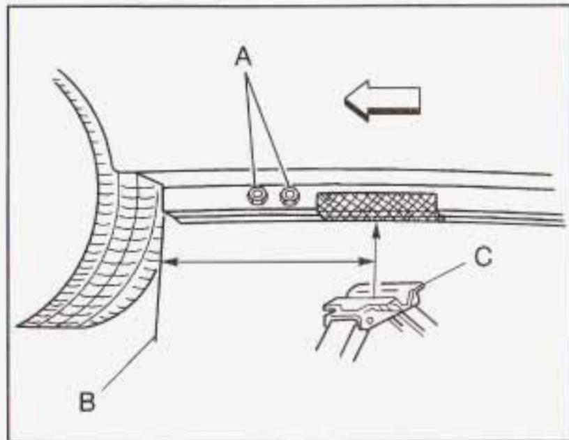
3. For jacking at the vehicle's front location, put the jack lift head (C) about 6 inches (15 cm) from the rear edge of the front wheel opening (B) or just behind the two bolts (A) as shown.
