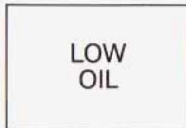
Your vehicle is equipped with an oil level monitoring system. When the ignition key is turned on, the LOW OIL light will come on briefly.
