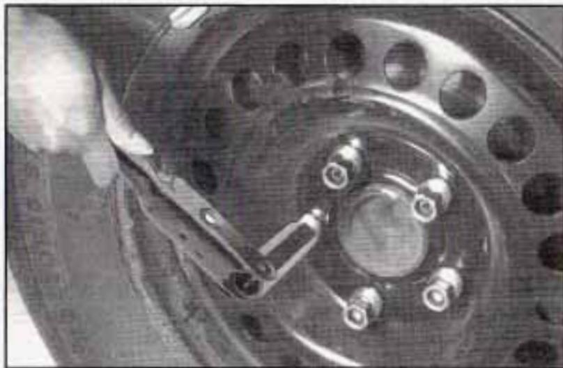
1. Using the wheel wrench, loosen all the wheel nuts. Don't remove them yet.
