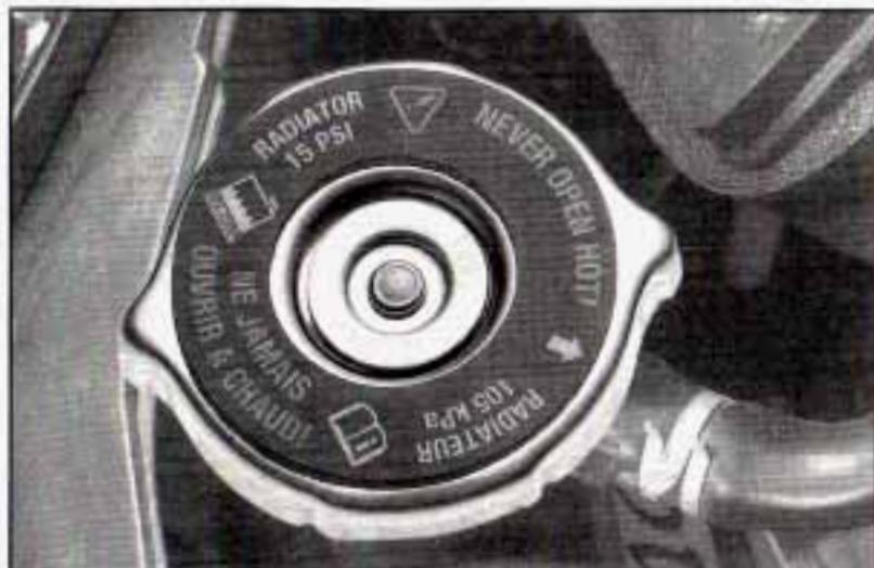
11. Then replace the pressure cap. At any time during this procedure if coolant begins to flow out of the filler neck, reinstall the pressure cap. Be sure the arrow on the pressure cap lines up like this.
