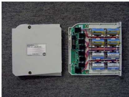
Example of incorporated batteries (Photo: 8 batteries incorporated)
