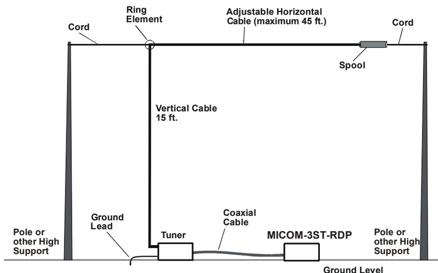
Figure 6. Erecting an Inverted "L" Long-Wire Antenna
