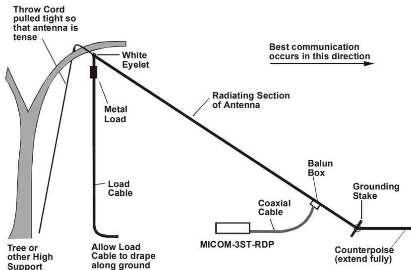
Figure 3. Erecting a Broadband Antenna with Earth Grounding
