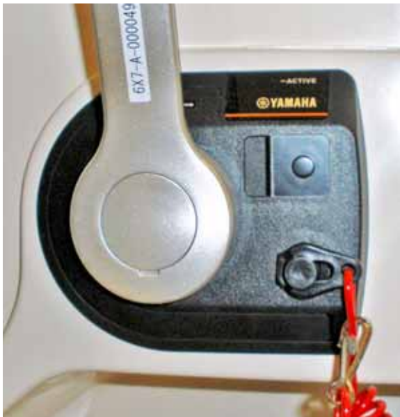
Engine Stop Switch
