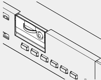
• If the SD card door does not close with a "click", check that the SD card is fully inserted into the slot.
