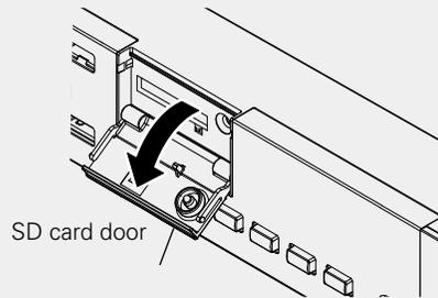
**2** Insert the SD card fully into the SD card slot until a "click" sound is heard.
