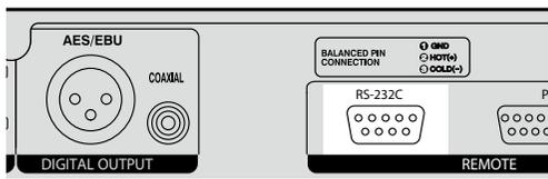
RS-232C control allows you to perform external control from the host. For details on RS-232C control, see "Serial remote control function" (page 56).
